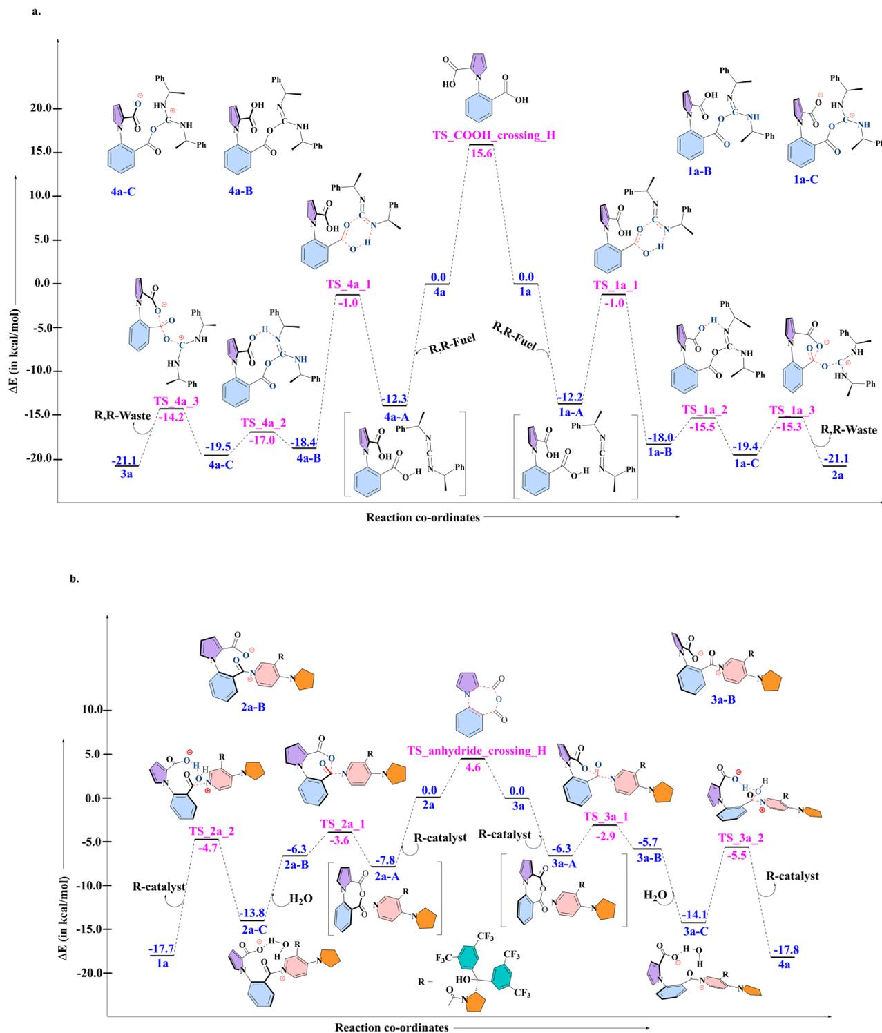
Fig. 6 The electronic energy values obtained from DFT, for the combination: **1a**, R, R-fuel, for the steps leading to (a) clockwise rotation (**1a** to **4a**), and anticlockwise rotation (**4a** to **1a**) and for the combination: **3a**, R-catalyst, for the steps leading to (b) clockwise rotation (**3a** to **4a**), and anticlockwise rotation (**2a** to **1a**).
