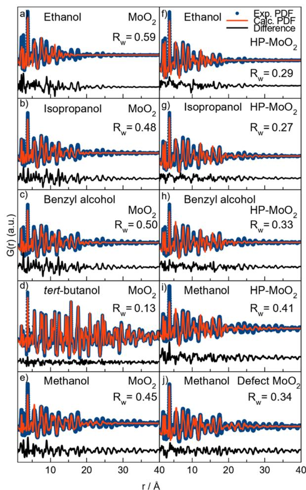
Fig. 3 PDFs obtained for MoO<sub>2</sub> synthesized at 200 °C in (a and f) ethanol, (b and g) isopropanol, (c and h) benzyl alcohol, (d) *tert*-butanol, and (e, i and j) methanol fitted with the distorted rutile MoO<sub>2</sub> structure and the high-pressure polymorph of MoO<sub>2</sub> as indicated. (j) Fitted with the distorted rutile MoO<sub>2</sub> structure with local point defects.
