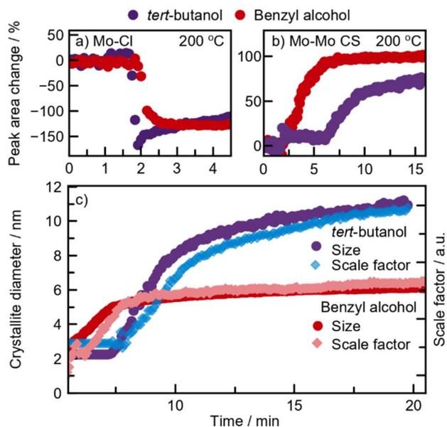
Fig. 6 Parameters extracted from *in situ* PDFs of  $\text{MoO}_2$  synthesized at 200 °C in *tert*-butanol and benzyl alcohol. Change of (a) Mo–Cl and (b) Mo–Mo CS peak area obtained from Gaussian fitting. (c) Crystallite sizes and scale factors determined from sequential PDF refinements.
