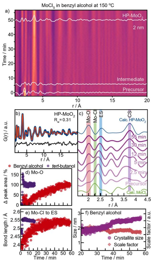
Fig. 7 HP- $\text{MoO}_2$  formation with benzyl alcohol at 150 °C. (a) Time-resolved PDFs. (b) PDF of final product fitted to HP- $\text{MoO}_2$ . (c) Selected PDFs throughout the reaction. (d) Change in the Mo–O peak area and (e) peak position from Gaussian fitting of PDFs during 150 °C syntheses in benzyl alcohol and *tert*-butanol. (f) Crystallite size and scale factor from sequential PDF refinements in benzyl alcohol. Refinement details are provided in Fig. S19.†
