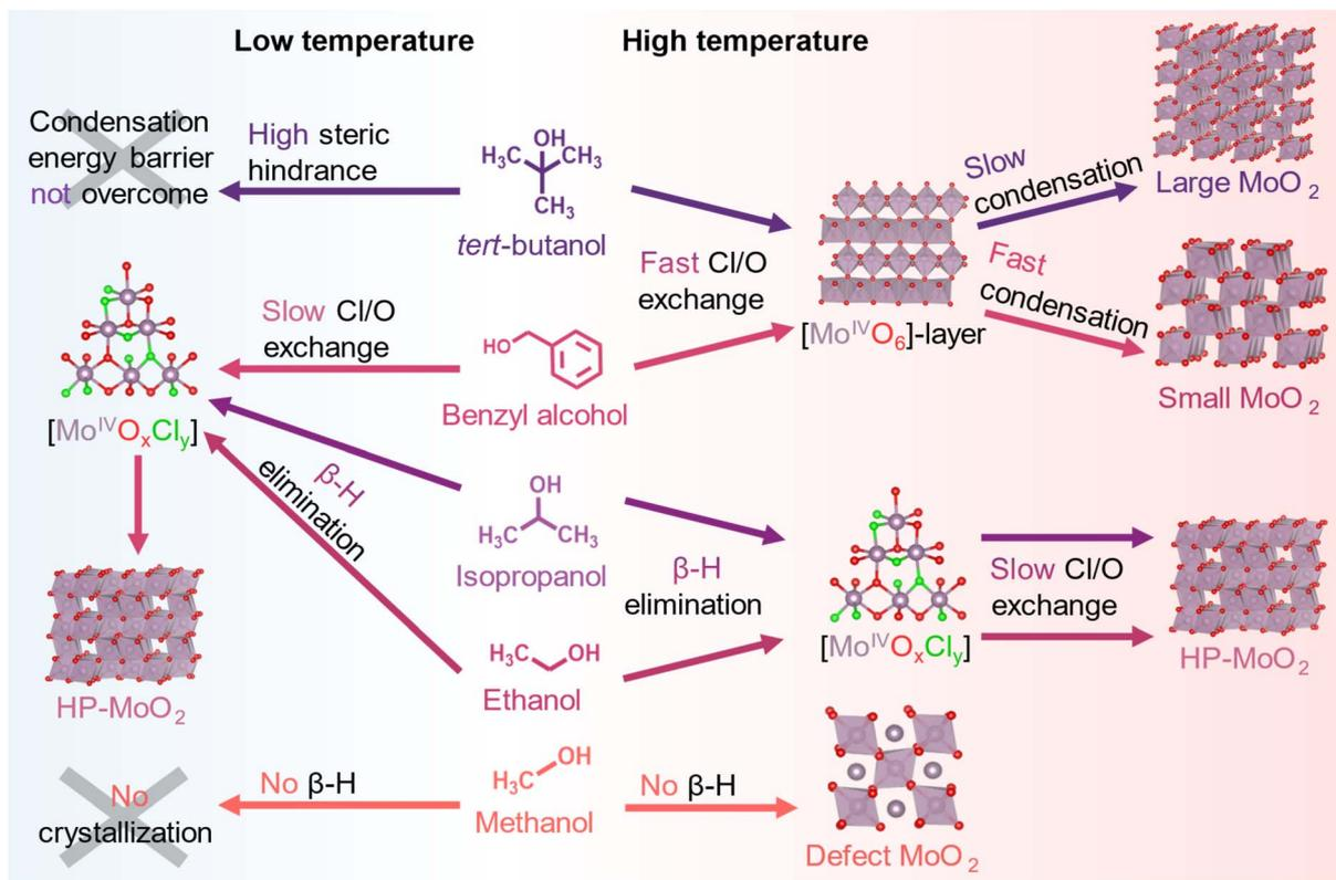
Fig. 9 Solvent influence in the solvothermal synthesis of MoO<sub>2</sub> polymorphs from MoCl<sub>5</sub> in methanol, ethanol, isopropanol, benzyl alcohol, or *tert*-butanol.
