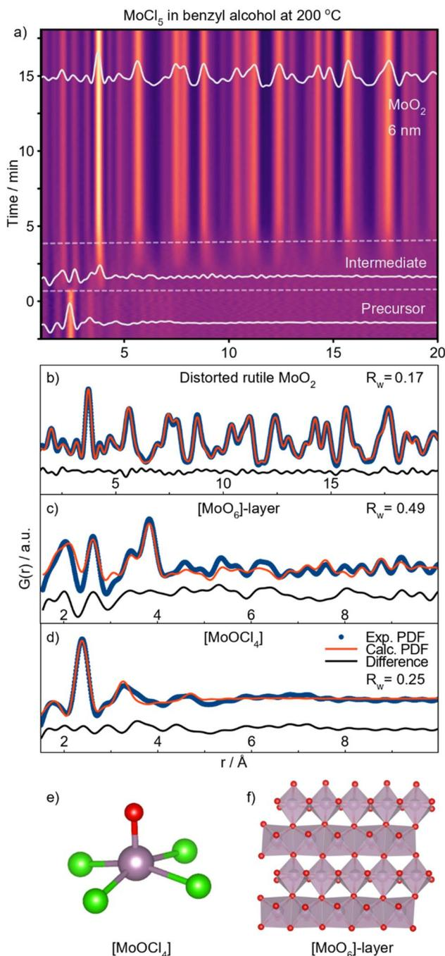
Fig. 5 Formation of distorted rutile MoO<sub>2</sub> using benzyl alcohol as solvent at 200 °C. (a) Time-resolved PDFs. (b) PDF of the final product fitted using distorted rutile MoO<sub>2</sub>. (c) Intermediate fitted with a layer of [MoO<sub>6</sub>]-octahedra (f). (d) Precursor PDF fitted with MoOCl<sub>4</sub> (e).
