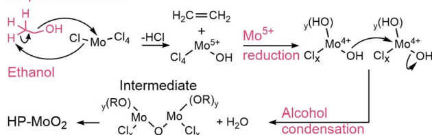
Scheme 3 Proposed E2 \beta -elimination reaction of MoCl_5 solvothermally treated in ethanol, followed by alcohol condensation. R = H, Mo.
