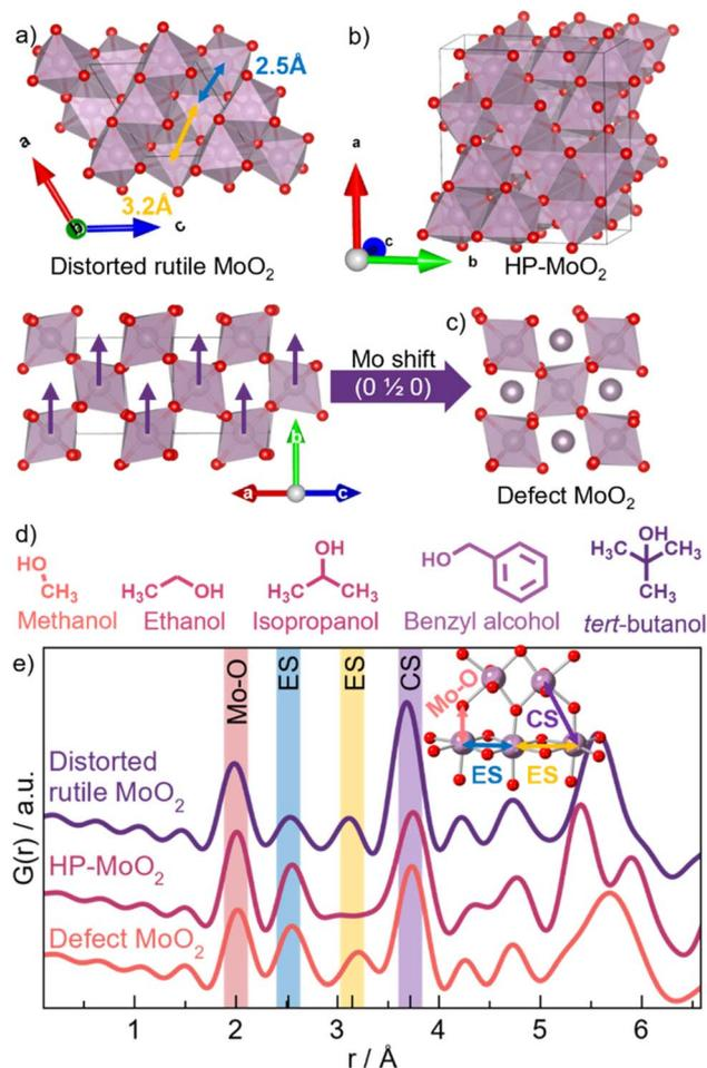
Fig. 1  $\text{MoO}_2$  structures. (a) Distorted rutile  $\text{MoO}_2$ . (b) HP- $\text{MoO}_2$ . (c) Defect  $\text{MoO}_2$  structure with additional Mo density in the interstitial sites of the distorted rutile structure. (d) Overview of solvents used. (e) Calculated PDFs from distorted rutile  $\text{MoO}_2$  (purple), HP- $\text{MoO}_2$  (pink), and defect  $\text{MoO}_2$  (orange) structures.
