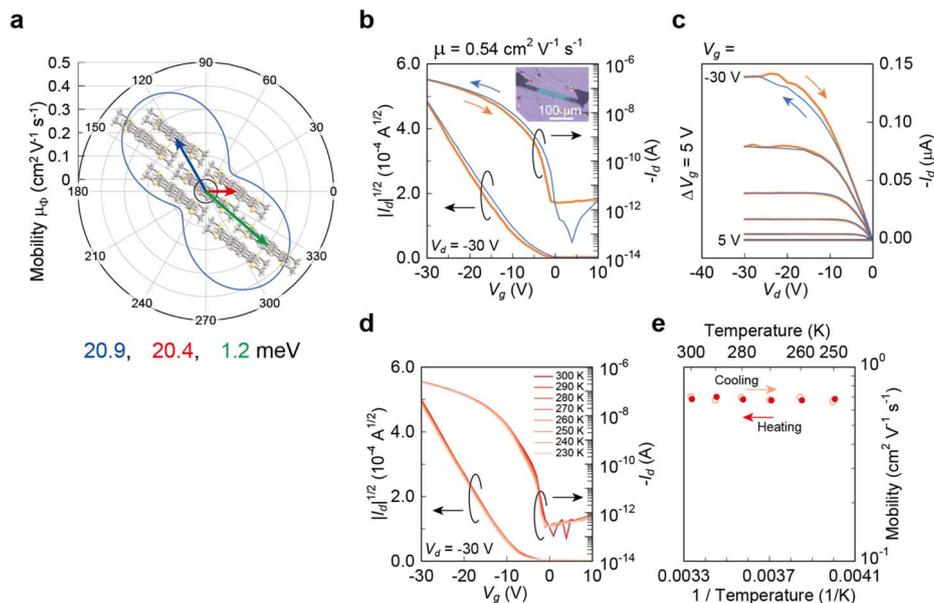
Fig. 3 Evaluation of MT-coronene as a semiconducting material. (a) Calculated  $t_s$  and estimated mobility based on the hopping model. (b) Transfer and (c) output characteristics of SC-FET of MT-coronene measured in air. (d) Transfer characteristics measured at various temperatures in a vacuum. (e) Temperature dependence of carrier mobility.
