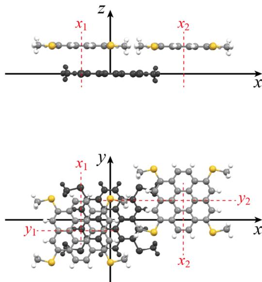
Fig. 4 Definition of mutual positions of molecules in the solid state. The first molecule (black in colour) is placed at the origin on the  $xy$ -plane of the Cartesian system so that the molecular long axis aligns with the  $x$ -axis, and the positions of the  $\pi$ -stacking molecules are defined by the coordinates of the center of gravity of the molecules. The  $y$ -axis projection (top) and the  $z$ -axis projection (bottom).
