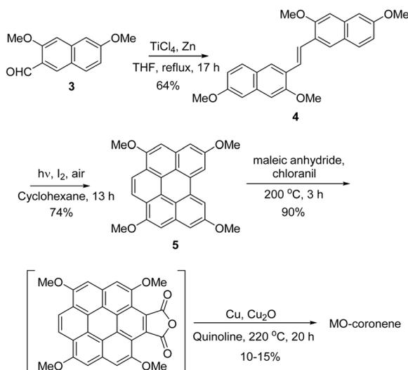
Scheme 2 Stepwise synthesis of MO-coronene from 2,7-dimethoxy-3-naphthaldehyde (**3**).
