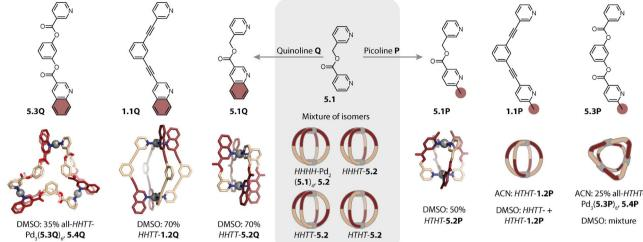
Fig. 20 Biasing the self-assembly of asymmetric ligands by introducing steric constraints on the donor site. (Left) For quinoline-equipped ligands the *HHTT*-isomer is favoured in DMSO. (Middle) Bis-pyridyl ligand **5.1** assembles to form a mixture of different isomers. (Right) For picolyl-equipped ligands, there is a bias towards *HTHT*-isomers.
