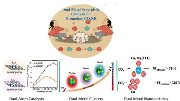
**Scheme 1** Different types of dual-metal catalysts with synergistic effects for promoting electrocatalytic CO<sub>2</sub> reduction. Reproduced with permission.<sup>124</sup> Copyright 2023, Elsevier. Reproduced with permission.<sup>96</sup> Copyright 2023, Wiley-VCH Verlag. Reproduced with permission.<sup>99</sup> Copyright 2024, John Wiley and Sons Ltd.
