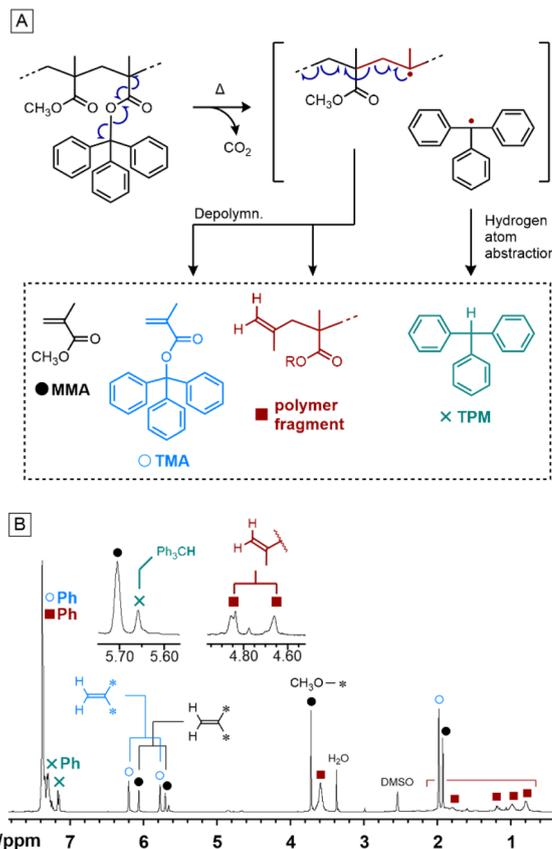
Fig. 3 (A) Proposal depolymerization-initiation mechanism for CPs with (B) <sup>1</sup>H NMR spectra (400 MHz, DMSO-d<sub>6</sub>, 25 °C) of the residue in the reactor after the monomer recovery test from **CP-5** at 270 °C within 15 min.
