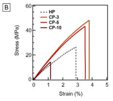
Fig. 4 (A) Transmittance of CP-5 and PMMA films. A photograph in the frame shows the cast film prepared from CP-5. (B) Stress—strain curves of the samples of poly(MMA-co-TMA)s and PMMA cut from their films pressed at 200 °C.
