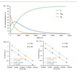
Fig. 6 (a) Concentration change of dihydroazaborinine 1, its corresponding intermediate  $\mathbf{1}_{IM}$  and Dewar isomer  $\mathbf{1}_{D}$  upon constant heating at 338 K for 10 h, (b) Arrhenius plot resulting from separate measurements at 333 K, 338 K, 343 K and 348 K. (c) Eyring plot resulting from separate measurements at 333 K, 338 K, 343 K and 348 K. RO: ring opening
