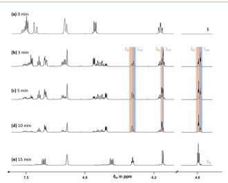
Fig. 5  $\,^{1}$ H NMR spectra of dihydroazaborinine **1** upon irradiation (280–400 nm) after (a) 0 min, (b) 3 min, (c) 5 min, (d) 10 min and (e) 15 min reveal stepwise photoisomerization process. Only the aromatic region as well as one additional Dewar signal (4.6 ppm) are shown for clarity. Full spectra can be found in the ESI.†
