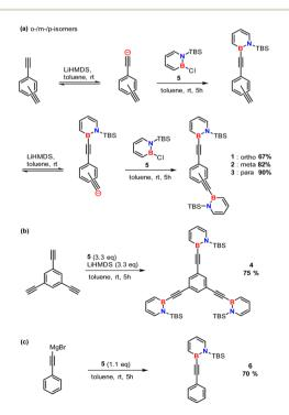
Scheme 1 Synthesis of (a) the high energy density dihydroazaborinines 1–3, (b) the trifold substituted species 4, and (c) the reference compound 6 with one dihydroazaborinine unit.
