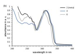
Fig. 4 Comparison of the UV-vis absorption spectra in cyclohexane (0.005–0.01 M, RT) of (a) the high energy density isomers 1–3 and (b) the *meta*-aligned high energy density dihydroazaborinines 2 and 4.
