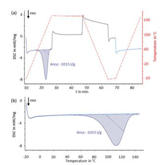
Fig. 8 DSC measurement of compound 4 including both heating gradients as well as the intermediate cooling in the device (b) and direct comparison of the first (dark blue) and second (light blue) heating plotted against the temperature.
