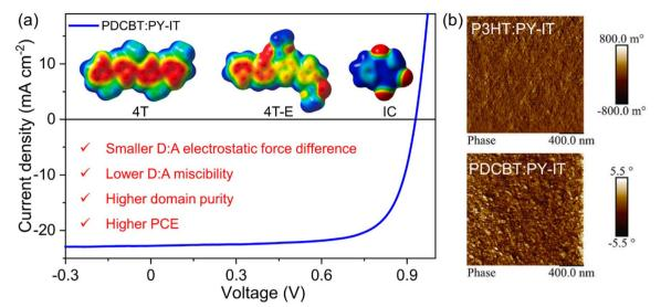
Fig. 12 (a) The electrostatic potential (ESP) distributions and device performance of PDCBT. (b) Atomic force microscopy (AFM) phase images of the P3HT:PY-IT and PDCBT:PY-IT blend films.<sup>115</sup>
