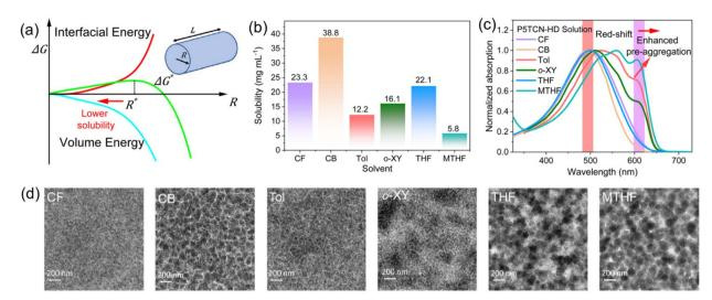
Fig. 10 (a) Schematic representation showing the dependence of Gibbs free energy of nucleation ( $\Delta G^*$ ) on the radius *R* according to classical nucleation theory; (b) the solubility of P5TCN-HD in different solvents; (c) normalized absorption spectra of P5TCN-HD in varied solvents. (d) Transmission electron microscopy (TEM) images of the blend films processed with different solvents.<sup>72</sup>
