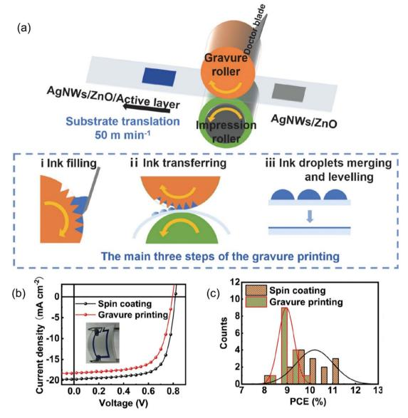
Fig. 13 (a) Schematic diagram of the fabrication of active layer films by gravure printing and the three main steps in the gravure process: (i) the doctor blade forces the ink to fill the gravure cavities; (ii) the ink is transferred from the cavities of the gravure roller to the substrate; (iii) ink droplets level on the substrate. (b) J-V curves and (c) efficiency statistical distributions of P5TCN-F25-based OSCs fabricated by spin-coated and gravure-printed active layers.147
