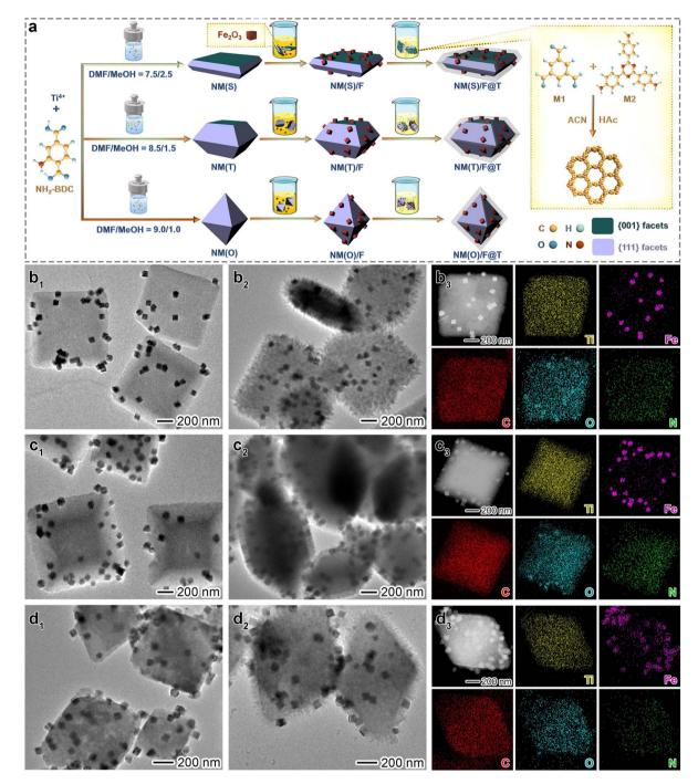
Fig. 1 Synthesis and electron microscopy characterization studies of NM/F and NM/F@T: (a) schematic illustration of the synthesis of NM/F and NM/F@T samples;  $(b_1-d_1)$  TEM images of  $(b_1)$  NM(S)/F,  $(c_1)$  NM(T)/F, and  $(d_1)$  NM(O)/F;  $(b_2-d_2)$  TEM,  $(b_3-d_3)$  STEM and EDS mapping images of  $(b_2)$  and  $(b_3)$  NM(S)/F@T,  $(c_2)$  and  $(b_3)$  NM(O)/F@T.
