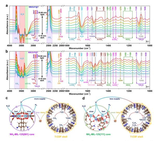
Fig. 6 Facet-dependent photocatalytic mechanisms of NM/F@T: (a and b) in situ DRIFTS of photocatalytic CO<sub>2</sub> reduction over (a) NM(S)/F@T and (b) NM(O)/F@T; (c and d) schematic illustration of the photocatalytic mechanisms of NM/F@T when NH2-MIL-125 is exposed with (c) {001} and (d) {111} facets.
