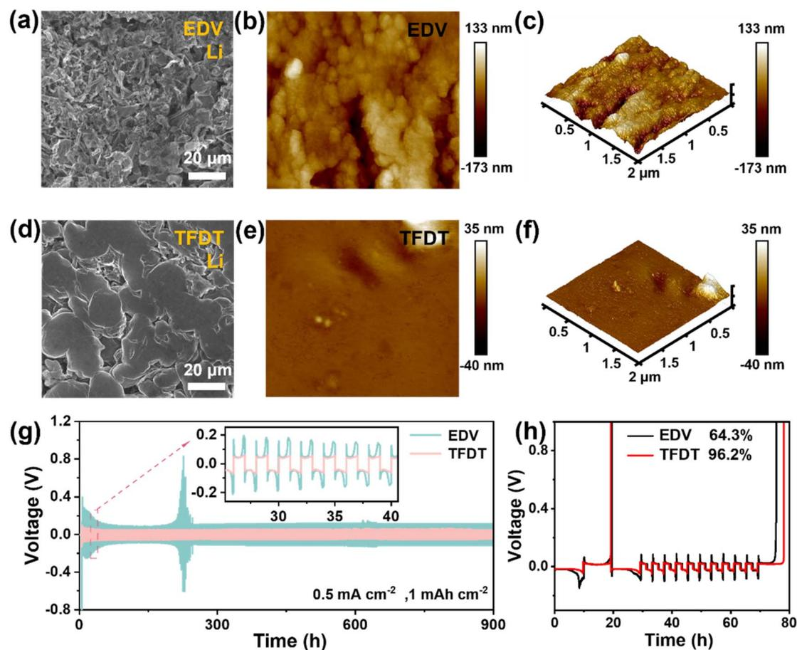
Fig. 3 SEM images of lithium metal anodes cycled in the electrolytes EDV (a) and TFDT (d) after 50 cycles at 1C with an upper charge cut-off voltage of 4.6 V in Li||LiCoO<sub>2</sub> coin cells. AFM images of lithium metal anodes cycled in EDV (b and c) and TFDT (e and f) under the same measurement conditions. (g) Plating/stripping voltage profiles of the Li||Li symmetrical cells in EDV and TFDT. (h) Voltage curves of plating/stripping for Li||Cu cells with EDV and TFDT.
