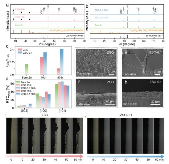
Fig. 5 Regulation of Zn deposition and suppression of dendritic growth. (a and b) XRD patterns of Zn electrodes before and after cycling in electrolytes. (c) Plots of the  $I_{(002)}/I_{(100)}$  ratio and (d) the RTC value. (e-h) SEM images of Zn anode after plating for 2 h at 1 mA cm<sup>-2</sup>. (i and j) *In situ* optical microscopy investigations of the Zn deposition in ZSO and ZSO-0.1 electrolytes at 1 mA cm<sup>-2</sup>.
