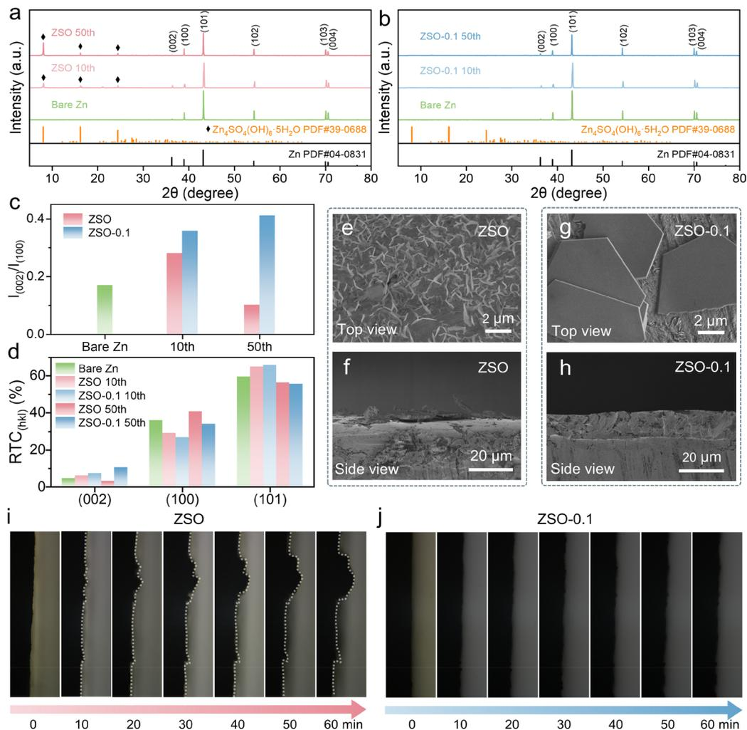
Fig. 5 Regulation of Zn deposition and suppression of dendritic growth. (a and b) XRD patterns of Zn electrodes before and after cycling in electrolytes. (c) Plots of the  $I_{(002)}/I_{(100)}$  ratio and (d) the RTC value. (e–h) SEM images of Zn anode after plating for 2 h at  $1 \text{ mA cm}^{-2}$ . (i and j) *In situ* optical microscopy investigations of the Zn deposition in ZSO and ZSO-0.1 electrolytes at  $1 \text{ mA cm}^{-2}$ .
