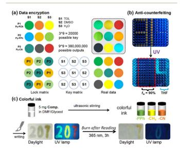
Fig. 9 Application examples of Py-R and Py-PR. (a) Solvent-based data encryption using Py-PCN, Py-PPh and Py-CN. (b) Fluorescent anti-counterfeiting using Py-Ph in THF and THF/H<sub>2</sub>O mixture ( $f_w = 90\%$ ) in a 384-well PCR plate. (c) Schematic illustration of the preparation and application of colourful fluorescent ink.
