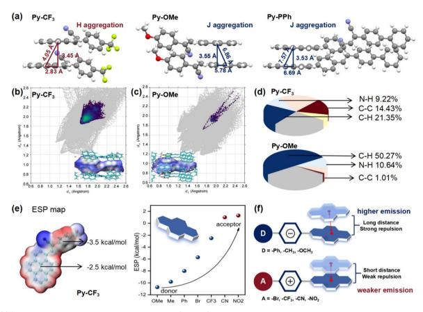
Fig. 5 (a) Single crystals and packing modes in dimers of  $Py-CF_3$ , Py-OMe, and Py-PPh; Hirshfeld surfaces and decomposed fingerprint plots of intermolecular C-C interaction of (b)  $Py-CF_3$  and (c) Py-OMe; (d) the contribution of various atoms in intermolecular interactions; (e) the molecular ESP of  $Py-CF_3$  and the variation of the ESP on pyrene with the end groups; (f) schematic illustration of aggregation mode influenced by the electronic effect of end groups.
