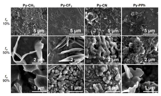
Fig. 4 SEM photographs of Py-CH<sub>3</sub>, Py-CF<sub>3</sub>, Py-CN and Py-PPh in a solution of THF/H<sub>2</sub>O with  $f_w = 10\%$ , 50% and 90%.
