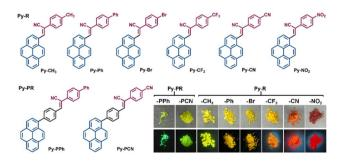
Fig. 1 The molecular structures of the  $\alpha$ -cyanostilbene pyrene-based molecules Py-R and Py-PR are illustrated. Insets show photographs of compounds Py-R and Py-PR under daylight (top) and UV irradiation (bottom).
