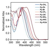
Fig. 2 UV-vis absorption spectra of Py-R and Py-PR in THF (10<sup>-5</sup> M).
