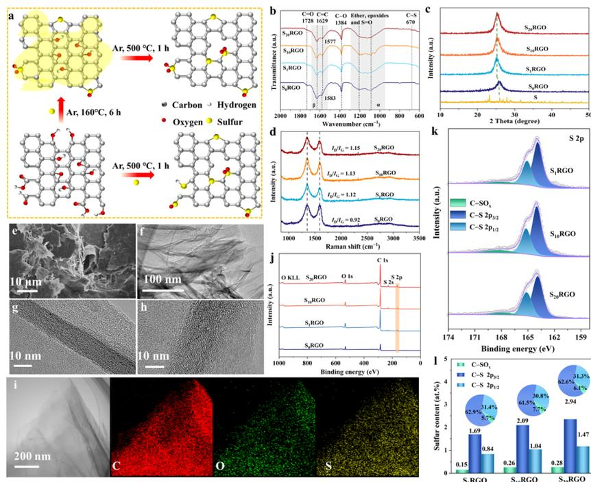
**Fig. 1** (a) Schematic illustration of the preparation of catalysts. (b) FTIR spectra, (c) XRD patterns, and (d) Raman spectra of  $S_x$ RGO. (e) SEM and (f) TEM of  $S_{10}$ RGO. HR-TEM images of (g)  $S_0$ RGO and (h)  $S_{10}$ RGO, and (i) element mapping of  $S_{10}$ RGO. (j) Survey XPS spectra of  $S_x$ RGO. (k) S 2p XPS spectra. (l) Proportional content of each sulfur configuration (inset is the sector diagram).
