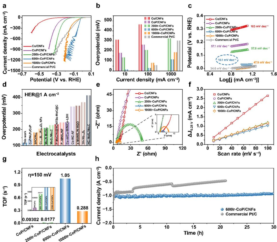
Fig. 3 HER tests in 0.5 M H<sub>2</sub>SO<sub>4</sub>. (a) LSV curves. (b) Overpotential comparison. (c) Tafel analysis. (d) Comparison of overpotentials at a current density of 1 A cm<sup>-2</sup> for various HER electrocatalysts with *iR*-correction. (e) Nyquist plots. (f) C<sub>dl</sub> value analysis. (g) TOF values. (h) *I*-*t* curves of 600Ir-CoP/CNFs and commercial Pt/C at ≈ 1 A cm<sup>-2</sup>.
