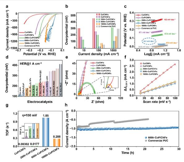
Fig. 3 HER tests in 0.5 M  $H_2SO_4$ . (a) LSV curves. (b) Overpotential comparison. (c) Tafel analysis. (d) Comparison of overpotentials at a current density of 1 A cm<sup>-2</sup> for various HER electrocatalysts with *iR*-correction. (e) Nyquist plots. (f)  $C_{dl}$  value analysis. (g) TOF values. (h) I-t curves of 600Ir-CoP/CNFs and commercial Pt/C at  $\approx$ 1 A cm<sup>-2</sup>.
