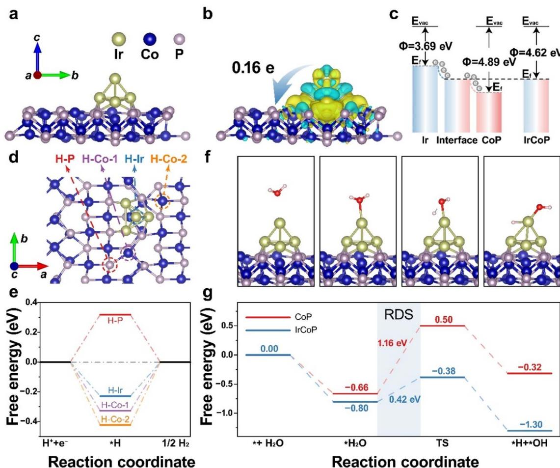
Fig. 5 DFT calculations of Ir–CoP and CoP for the HER. (a) The model of Ir–CoP. (b) Charge density of Ir–CoP, indicating electron gain (yellow) and loss (blue). (c) The work function of Ir, CoP, and Ir–CoP. (d) Sites of  $*H$  adsorption on the Ir–CoP model. (e)  $\Delta G_{H^*}$  on varied adsorption sites. (f) Intermediate adsorption configurations of water dissociation on Ir–CoP. (g) The kinetic barrier of water dissociation on Ir–CoP and CoP.
