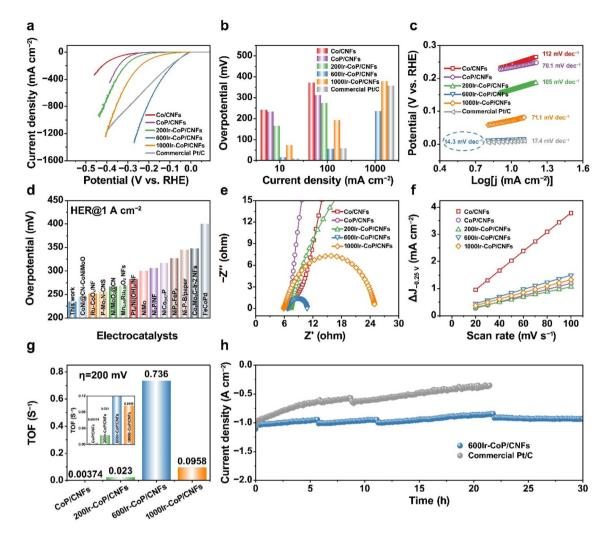
Fig. 4 HER tests in 1.0 M KOH. (a) LSV curves. (b) Overpotential comparison. (c) Tafel analysis. (d) Comparison of overpotentials at a current density of 1.0 A cm<sup>-2</sup> for various HER electrocatalysts with iR-correction. (e) Nyquist plots. (f) C<sub>dl</sub> values. (g) TOF values. (h) I-t curves of 600Ir-CoP/CNFs and commercial Pt/C at  $\approx 1 \text{ A cm}^{-2}$
