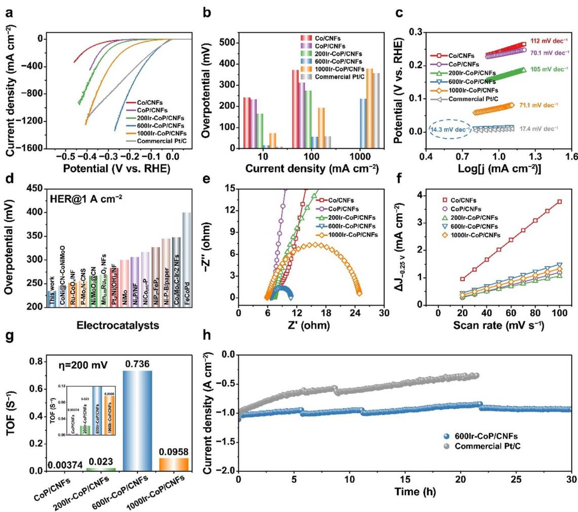
Fig. 4 HER tests in 1.0 M KOH. (a) LSV curves. (b) Overpotential comparison. (c) Tafel analysis. (d) Comparison of overpotentials at a current density of  $1.0 \text{ A cm}^{-2}$  for various HER electrocatalysts with  $iR$ -correction. (e) Nyquist plots. (f)  $C_{dl}$  values. (g) TOF values. (h)  $I-t$  curves of 600Ir-CoP/CNFs and commercial Pt/C at  $\approx 1 \text{ A cm}^{-2}$ .
