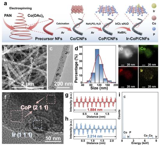
Fig. 1 (a) Synthetic route illustration for Ir–CoP/CNFs. (b) SEM, (c) TEM, and (d) diameter distribution of 600Ir–CoP/CNFs. (e) Elemental mapping of Co, P, and Ir elements of 600Ir–CoP/CNFs. (f) HRTEM image of 600Ir–CoP/CNFs. FFT-based crystal plane spacing distribution histogram of (g) CoP (211) and (h) Ir (111). (i) EDX spectrum of 600Ir–CoP/CNFs.
