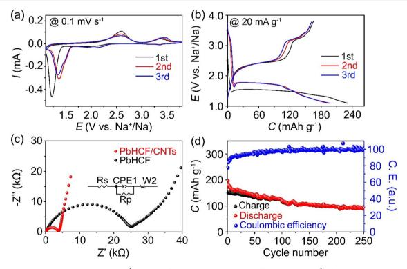
Fig. 3 (a) CV curves of PbHCF/CNTs at  $0.1 \, \text{mV s}^{-1}$ ; (b) charge/discharge curves of PbHCF/CNTs at 20 mA  $g^{-1}$ ; (c) EIS curves of both PbHCF/CNTs and PbHCF; (d) cycling performance at 100 mA  $g^{-1}$  of PbHCF/CNTs in SIBs.
