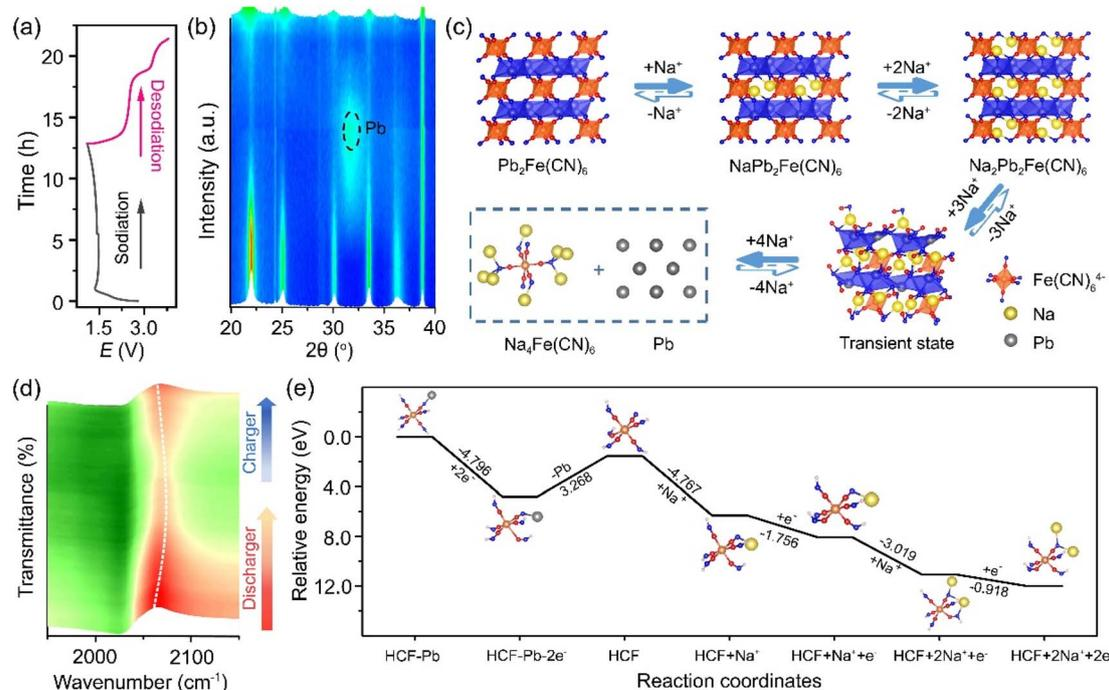
Fig. 4 (a) Charge/discharge curves of PbHCF/CNTs at 20  $\text{mA g}^{-1}$ ; (b) *operando* XRD results of PbHCF/CNTs during the first cycle; (c) schematic diagram of redox mechanism of PbHCF/CNTs cathode materials; (d) *in situ* FTIR contour map of PbHCF/CNTs during the first cycle; (e) schematic diagram of energy changes during discharging processes.
