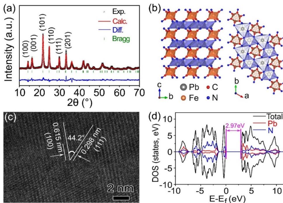
Fig. 1 (a) Structural refinement of XRD patterns of PbHCF/CNTs; (b) crystal structure of PbHCF consisting of layer structure with  $\text{PbN}_6$  (blue) and  $\text{FeC}_6$  (orange) polyhedra; (c) HRTEM image of PbHCF/CNTs; and (d) DOS of PbHCF.
