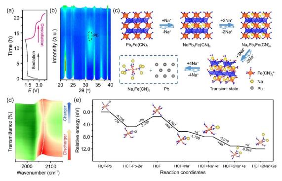
Fig. 4 (a) Charge/discharge curves of PbHCF/CNTs at 20 mA  $g^{-1}$ ; (b) operando XRD results of PbHCF/CNTs during the first cycle; (c) schematic diagram of redox mechanism of PbHCF/CNTs cathode materials; (d) in situ FTIR contour map of PbHCF/CNTs during the first cycle; (e) schematic diagram of energy changes during discharging processes.
