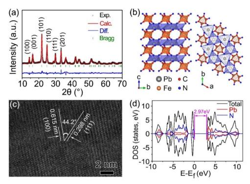
Fig. 1 (a) Structural refinement of XRD patterns of PbHCF/CNTs; (b) crystal structure of PbHCF consisting of layer structure with PbN<sub>6</sub> (blue) and  $FeC_6$  (orange) polyhedra; (c) HRTEM image of PbHCF/CNTs; and (d) DOS of PbHCF.
