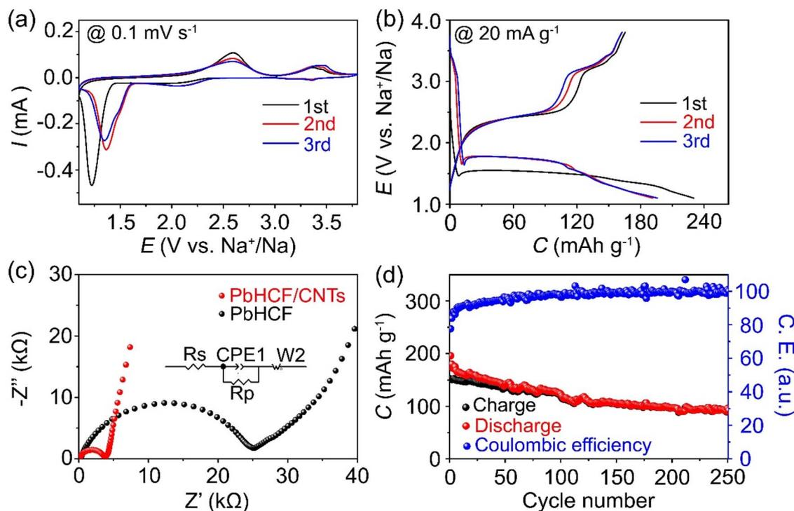
Fig. 3 (a) CV curves of PbHCF/CNTs at  $0.1 \text{ mV s}^{-1}$ ; (b) charge/discharge curves of PbHCF/CNTs at  $20 \text{ mA g}^{-1}$ ; (c) EIS curves of both PbHCF/CNTs and PbHCF; (d) cycling performance at  $100 \text{ mA g}^{-1}$  of PbHCF/CNTs in SIBs.
