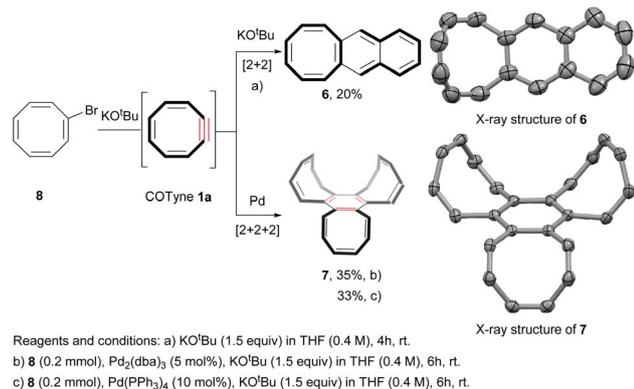
**Scheme 2** Transition-metal free and Pd-catalyzed cycloadditions of COTyene **1a**. ORTEP drawing of naphthoCOT **6** and benzotri[8]annulene **7** showing thermal ellipsoids at the 50% probability level, H atoms have been omitted for clarity.
