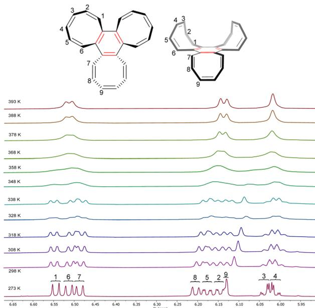
Fig. 2 VT-<sup>1</sup>H NMR spectra of ( $\alpha,\alpha,\beta$ )-benzotri[8]annulene 7.
