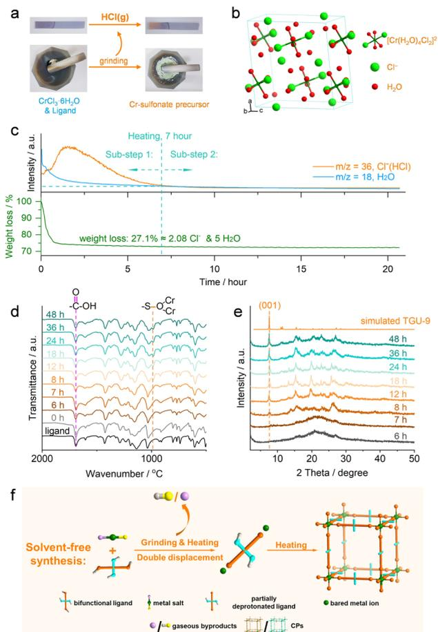
Fig. 5 Solvent-free synthesis mechanism analysis of Cr(III)-sulfonate frameworks. (a) Visualized detection of HCl gas during the grinding of CrCl<sub>3</sub>·6H<sub>2</sub>O and the NAP(COOH)<sub>2</sub>(SO<sub>3</sub>H)<sub>2</sub> ligand. (b) Unit cell of CrCl<sub>3</sub>·6H<sub>2</sub>O. (c) Time-dependent TG-MS spectra during the heating step. (d and e) Time-dependent PXR patterns and FT-IR spectra of the crude TGU-9, respectively. (f) Proposed solvent-free synthesis mechanism.
