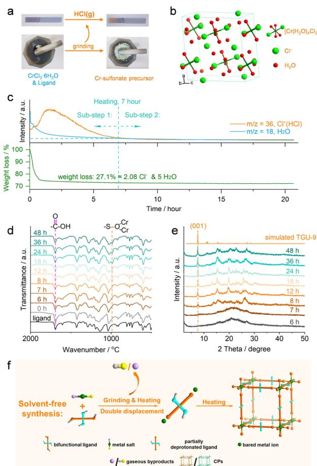
Fig. 5 Solvent-free synthesis mechanism analysis of Cr(III)-sulfonate frameworks. (a) Visualized detection of HCl gas during the grinding of CrCl<sub>3</sub>·6H<sub>2</sub>O and the NAP(COOH)<sub>2</sub>(SO<sub>3</sub>H)<sub>2</sub> ligand. (b) Unit cell of CrCl<sub>3</sub>·6H<sub>2</sub>O. (c) Time-dependent TG-MS spectra during the heating step. (d and e) Time-dependent PXRD patterns and FT-IR spectra of the crude TGU-9, respectively. (f) Proposed solvent-free synthesis mechanism.
