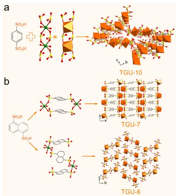
Fig. 4 Tuned Cr–SO<sub>3</sub> coordination under solvent-free conditions. (a) TGU-10 consisted of BDS<sup>2−</sup> linkers and Cr<sub>2</sub>(SO<sub>3</sub>)<sub>6</sub>(H<sub>2</sub>O)<sub>4</sub> SBUs. (b) TGU-7 and TGU-8 supramolecular frameworks constructed by NDS<sup>2−</sup> linkers and different 0D Cr–SO<sub>3</sub> clusters.
