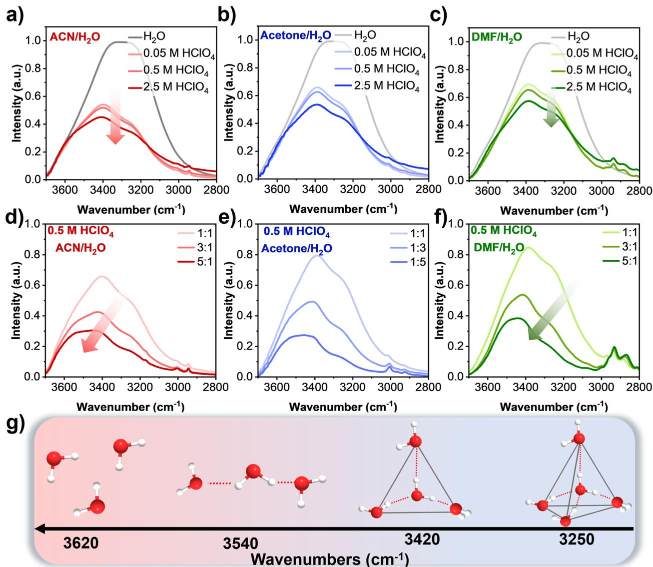
Fig. 5 (a)–(c) FTIR spectra of organic solvent/water mixtures with different  $\text{HClO}_4$  concentrations. (d)–(f) FTIR spectra of 0.5 M  $\text{HClO}_4$  organic solvent/water mixtures with different volume ratios of solvent and water (1 : 1, 3 : 1 and 5 : 1). (g) Scheme of the change in water structures with different electrolyte compositions.
