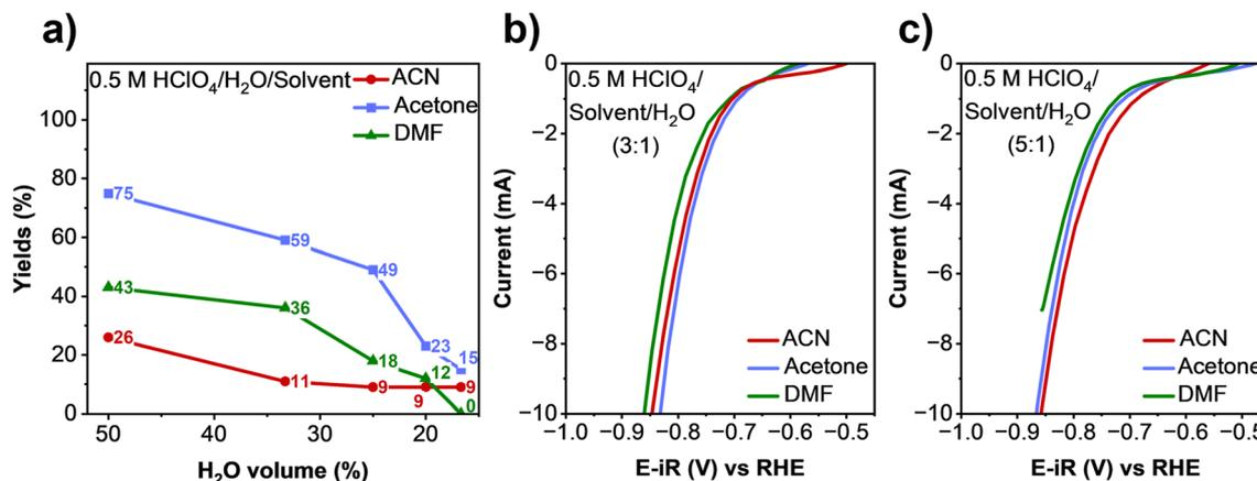
Fig. 2 (a) Yields in the 0.5 M HClO<sub>4</sub> hybrid electrolytes with different H<sub>2</sub>O and organic solvent compositions. (b) and (c) Cyclic voltammograms recorded for hybrid electrolytes containing 0.5 M HClO<sub>4</sub> with different H<sub>2</sub>O and organic solvent compositions.
