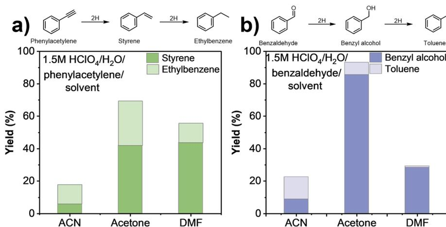
Fig. 3 The yield of electrochemical semihydrogenation of (a) phenylacetylene and (b) benzaldehyde at  $-1.1$  vs. RHE in 1.5 M HClO<sub>4</sub>/H<sub>2</sub>O/DMF hybrid electrolytes for 2 hours using Ni foam.
