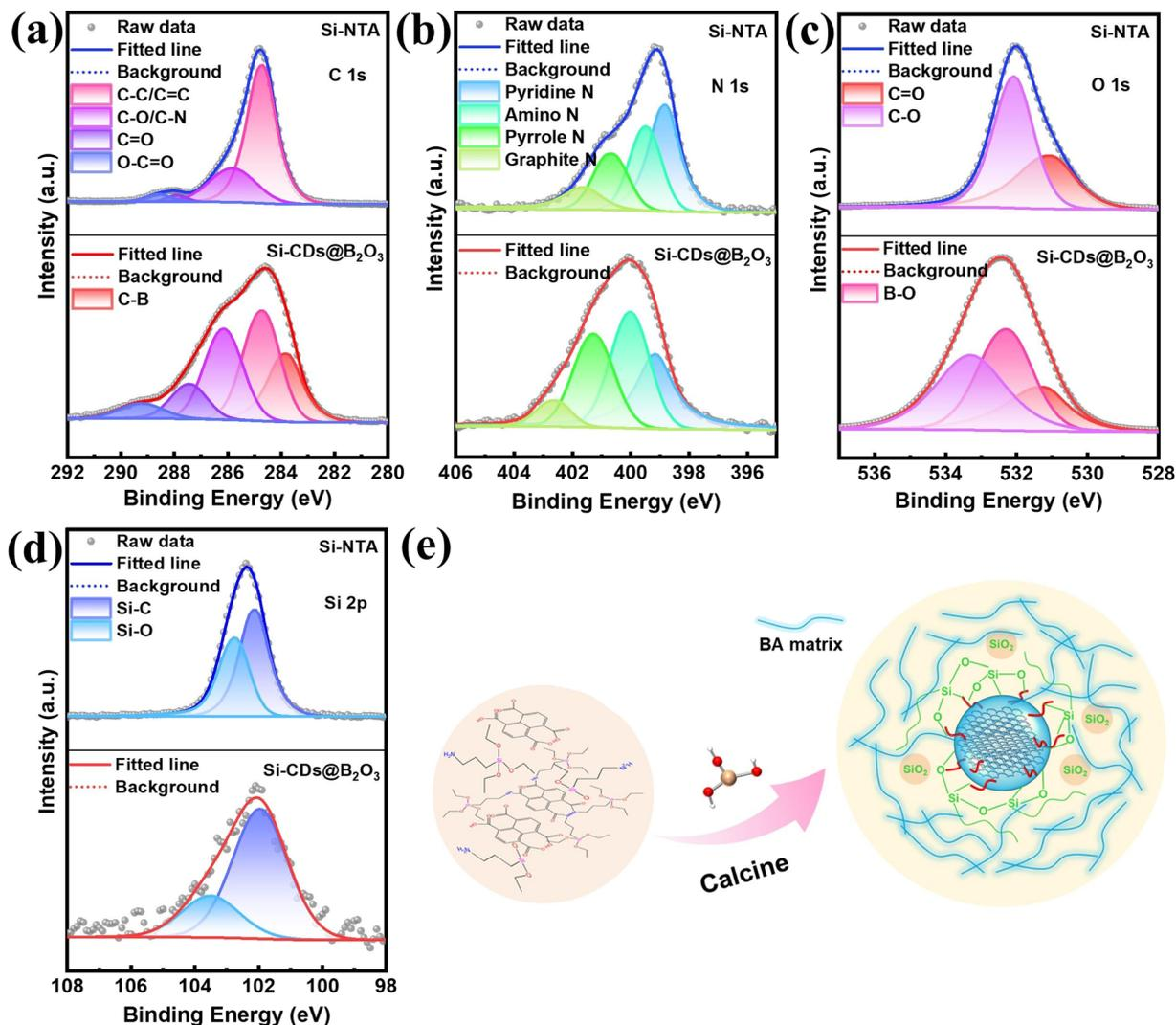
Fig. 2 (a–d) High-resolution C 1s, N 1s, O 1s and Si 2p spectra of Si-NTA and Si-CDs@B<sub>2</sub>O<sub>3</sub>. (a) C 1s, (b) N 1s, (c) O 1s, and (d) Si 2p. (e) Schematic diagram of the Si-CDs@B<sub>2</sub>O<sub>3</sub> composite network structure before and after calcination.
