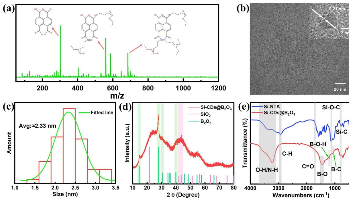
Fig. 1 (a) The HR-MS spectrum of the Si-NTA. (b) The TEM and HR-TEM image of Si-CDs@B<sub>2</sub>O<sub>3</sub>. (c) The particle size distribution of Si-CDs@B<sub>2</sub>O<sub>3</sub>. (d) The XRD spectra of Si-CDs@B<sub>2</sub>O<sub>3</sub> (SiO<sub>2</sub>, PDF#27-0605; B<sub>2</sub>O<sub>3</sub>, PDF#06-0297). (e) The FT-IR spectra of Si-NTA and Si-CDs@B<sub>2</sub>O<sub>3</sub>.
