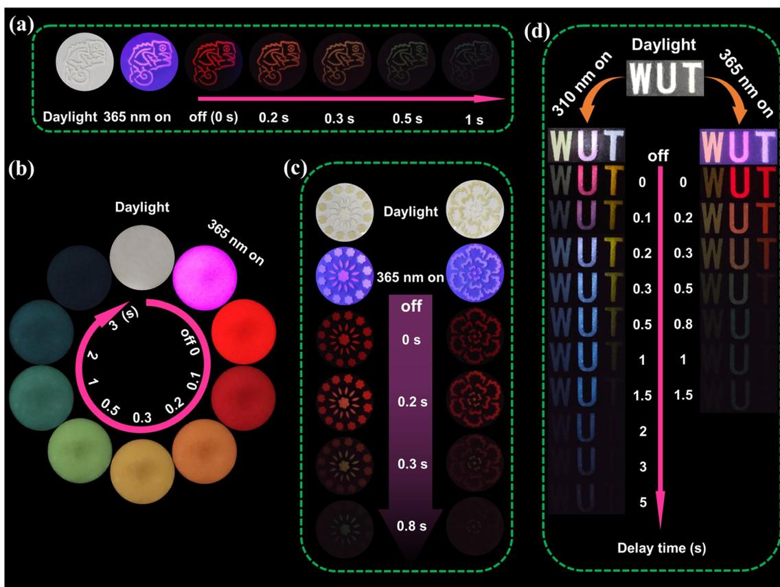
Fig. 4 (a) Optical photographs of the chameleon pattern after 365 nm irradiation. (b) Optical photographs of Si-CDs@B<sub>2</sub>O<sub>3</sub> composites after 365 nm irradiation. (c) Optical photographs of the flower pattern after 365 nm irradiation. (d) Images of the “WUT” letter under 310 nm and 365 nm irradiation on and off.
