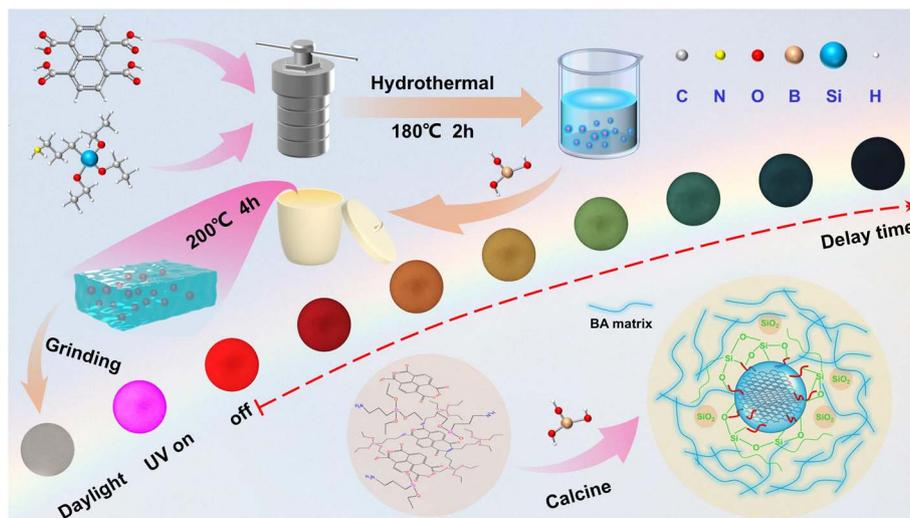
Scheme 1 Schematic diagram of the synthesis, structure and phosphorescence properties of Si-CDs@B<sub>2</sub>O<sub>3</sub>.
