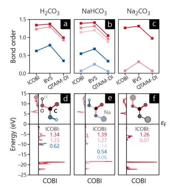
Fig. 6 Bond orders of (a) H<sub>2</sub>CO<sub>3</sub>, (b) NaHCO<sub>3</sub> and (c) Na<sub>2</sub>CO<sub>3</sub> as well as energy-resolved crystal orbital bond indices of (d) H<sub>2</sub>CO<sub>3</sub>, (e) NaHCO<sub>3</sub> and (f) Na<sub>2</sub>CO<sub>3</sub>. The color codes of the bond orders in (a)–(c) correspond to the color-coded bonds in (d)-(f)
