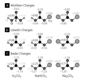
Fig. 5 Simplified depictions of solid-state carbonic acid, sodium hydrogen carbonate and sodium carbonate with the corresponding (a) Mulliken and (b) Löwdin charges as calculated using LOBSTER. Bader charges are provided in (c) for comparison.
