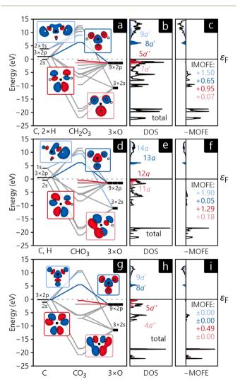
Fig. 9 Molecular orbital diagram (a, d and g), MO-projected density of states (b, e and h) and molecular orbital formation energy MOFE (c, f and i) for  $H_2CO_3$  (a–c),  $HCO_3^-$  (d–f), and  $CO_3^{2-}$  (g–i). IMOFE is given in eV.
