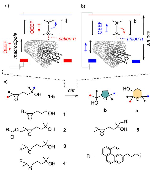
Fig. 1 (a) Electric-field cation- $\pi$  and (b) anion- $\pi$  catalysis to cleave the bond X–Y on MWCNTs in electromicrofluidic devices (OEEF = oriented external electric field). (c) Structure of previous (1) and new substrates (2–5) and products a (anti-Baldwin) and b (Baldwin) of epoxide-opening ether cyclization.
