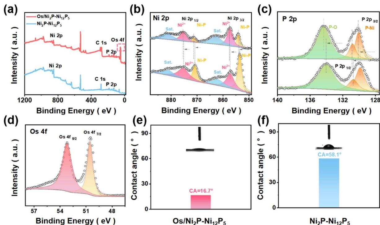
Fig. 2 (a) XPS spectra of Os/Ni<sub>2</sub>P–Ni<sub>12</sub>P<sub>5</sub> and Ni<sub>2</sub>P–Ni<sub>12</sub>P<sub>5</sub>. (b) Ni 2p, (c) P 2p, and (d) Os 4f. The water contact angle measurements of (e) Ni<sub>2</sub>P–Ni<sub>12</sub>P<sub>5</sub> and (f) Os/Ni<sub>2</sub>P–Ni<sub>12</sub>P<sub>5</sub>.
