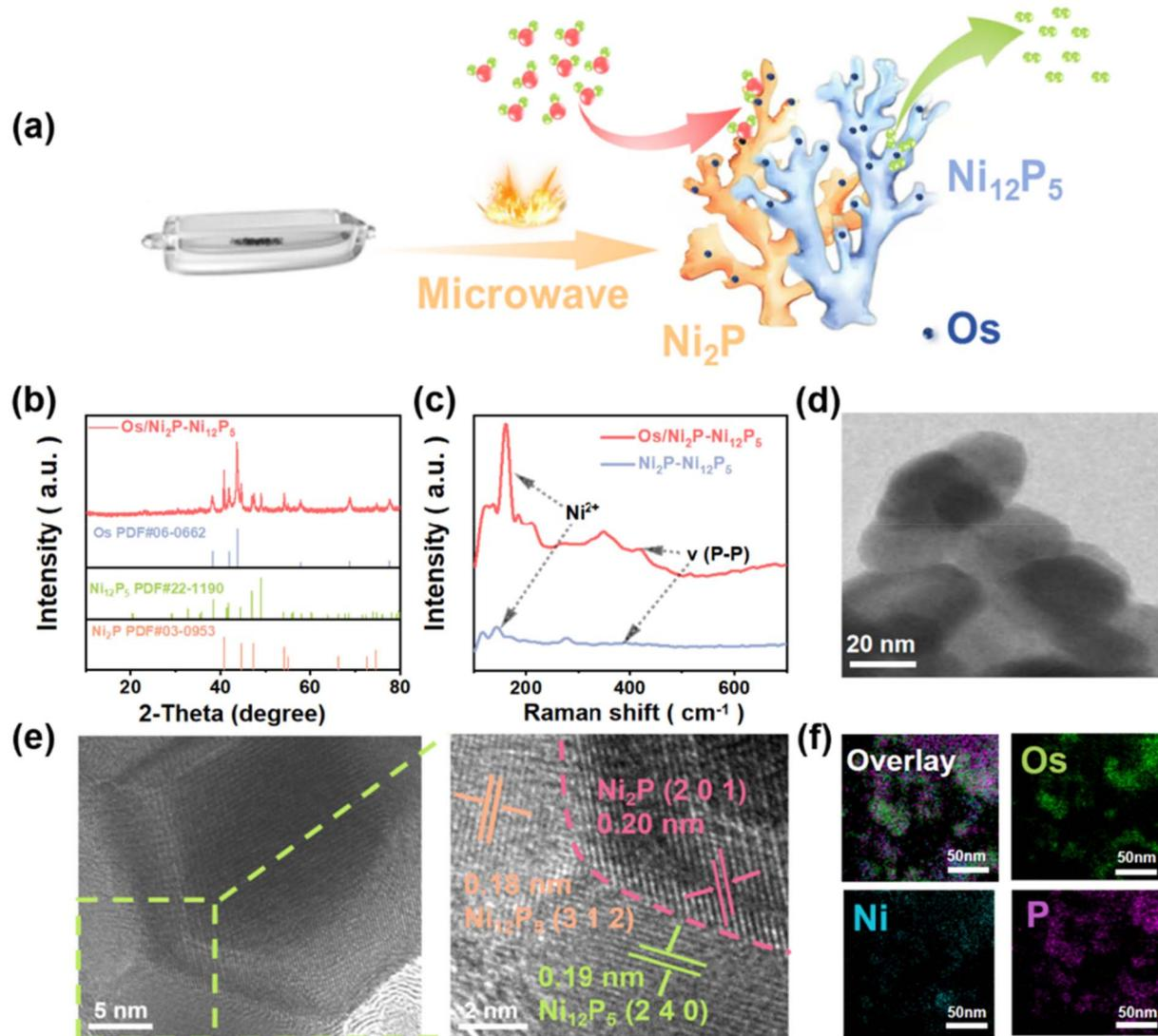
Fig. 1 (a) Schematic diagram of the preparation process for Os/Ni<sub>2</sub>P–Ni<sub>12</sub>P<sub>5</sub>. (b) XRD pattern. (c) Raman spectra. (d) TEM image and (e) HRTEM image of Os/Ni<sub>2</sub>P–Ni<sub>12</sub>P<sub>5</sub>. (f) EDS elemental mappings for Os/Ni<sub>2</sub>P–Ni<sub>12</sub>P<sub>5</sub>.
