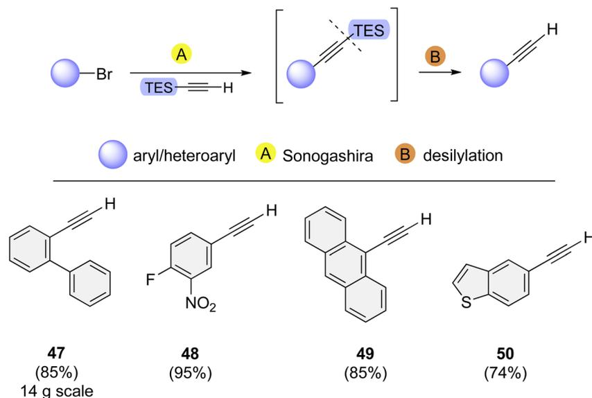
**Scheme 4** Synthetic approach to terminal alkynes using **L4** as the ligand; reaction conditions: step A: aryl bromide (1 equiv.), TES acetylene (1.2 equiv.), Pd(OAc)<sub>2</sub> (0.5 mol%), **L4** (2 mol%), NEt<sub>3</sub> (3 equiv.), 2 wt% SDS/H<sub>2</sub>O (0.5 M), CPME (20 v/v%), 70 °C, Ar, 16 h. Step B: TBAF (1 M in THF, 1.5 equiv.), DCM (0.1 M), 0 °C to rt, 2 h.
