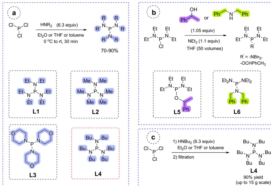
**Scheme 1** (a) Different variations of synthesized symmetrical aminophosphines. (b) Unsymmetrical variation of aminophosphines. (c) Scaled-up synthesis of **L4**.
