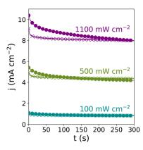
Fig. 7 CA measurements of a 50% omission electrode in 0.1 M KOH at  $E=1.7~\rm V~vs.$  RHE under various illumination intensities from a 365 nm LED. Lines with solid circles indicate illumination from the front side of the electrode, and lines with '×' indicate illumination from the back side of the electrode.
