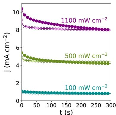
Fig. 7 CA measurements of a 50% omission electrode in 0.1 M KOH at  $E = 1.7$  V vs. RHE under various illumination intensities from a 365 nm LED. Lines with solid circles indicate illumination from the front side of the electrode, and lines with 'x' indicate illumination from the back side of the electrode.
