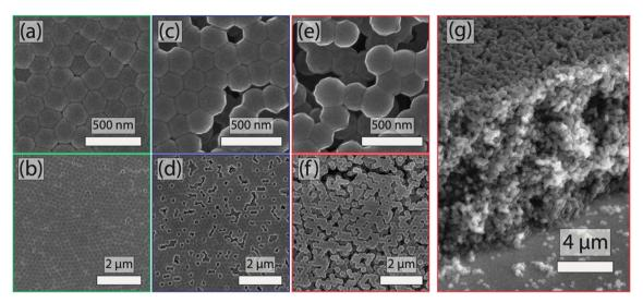
Fig. 1 Scanning electron micrographs of a 0% (a and b), a 20% (c and d), and a 50% (e and f) omission glass photoelectrode composed of 200 nm  $SiO_2$  nanospheres and a 20 nm layer of  $TiO_2$ . (g) A side-on image of the 50% omission glass photoelectrode, indicating that the structure was roughly 15  $\mu$ m thick.
