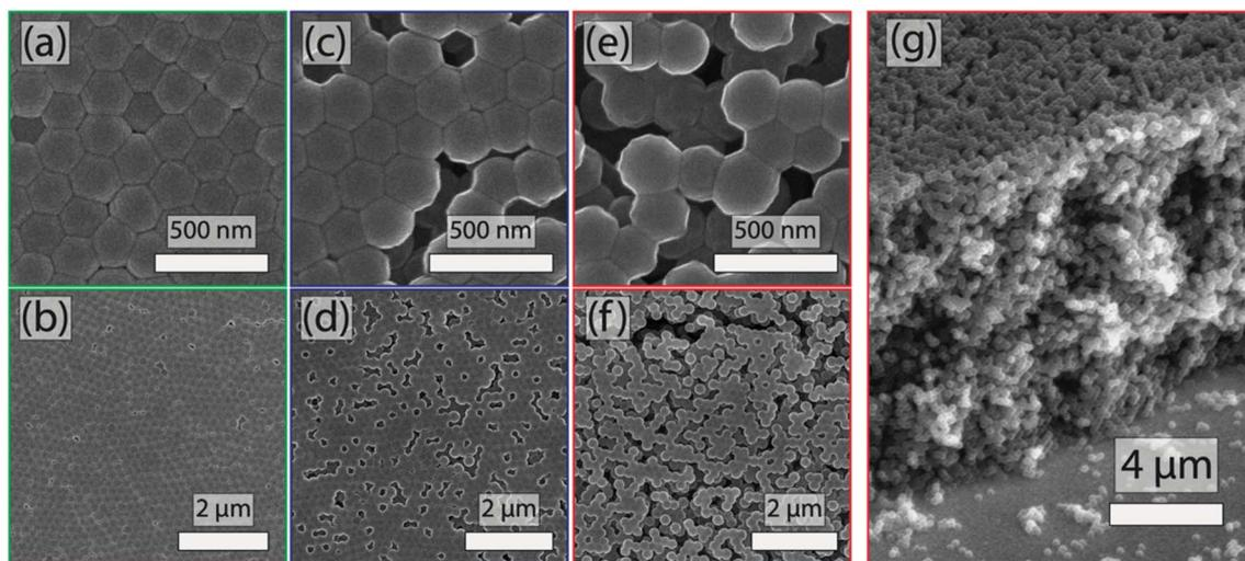
**Fig. 1** Scanning electron micrographs of a 0% (a and b), a 20% (c and d), and a 50% (e and f) omission glass photoelectrode composed of 200 nm SiO<sub>2</sub> nanospheres and a 20 nm layer of TiO<sub>2</sub>. (g) A side-on image of the 50% omission glass photoelectrode, indicating that the structure was roughly 15 μm thick.
