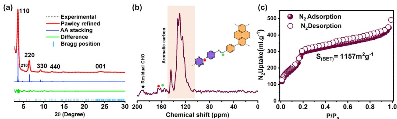
Fig. 1 (a) PXRD patterns of **Py-Tz** COF; experimental obtained (dotted black), Pawley refined (red), simulated pattern for AA stacking (blue) and their difference (green). (b) Solid-state <sup>13</sup>C NMR spectra of **Py-Tz** COF. (c) N<sub>2</sub> sorption isotherm of **Py-Tz** COF measured at 77 K.
