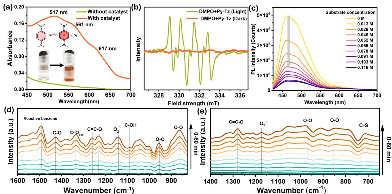
Fig. 3 (a) UV-vis spectra of TMPD radical cation formed by Py-Tz COF in the presence of light and  $O_2$ . (b) EPR spectra of  $DMPO-O_2^-$  formed by Py-Tz COF in the presence of light. (c) Photoluminescence quenching experiment of Py-Tz COF in THF dispersion by varying concentrations of  $N,N$ -dimethylaniline. *In situ* DRIFT studies demonstrate the appearance of new peaks, showing the progression of (d) hydroxylation reaction and (e) thiocyanation reaction.
