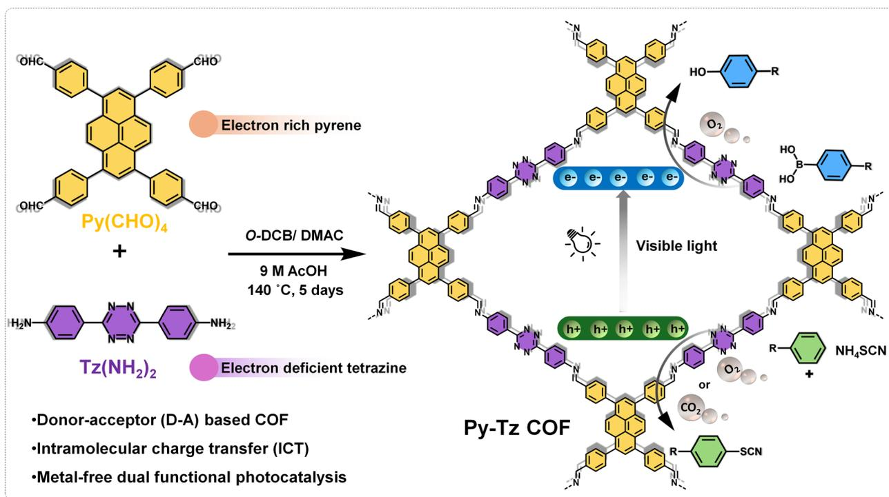
Scheme 1 Synthetic scheme of donor–acceptor **Py-Tz** COF from Py(CHO)<sub>4</sub> and Tz(NH<sub>2</sub>)<sub>2</sub>, serving as a metal-free dual-functional heterogeneous photocatalyst. Two different organic transformation reactions: e<sup>−</sup>-catalysed hydroxylation and h<sup>+</sup>-catalysed thiocyanation reactions conducted in a single pot.
