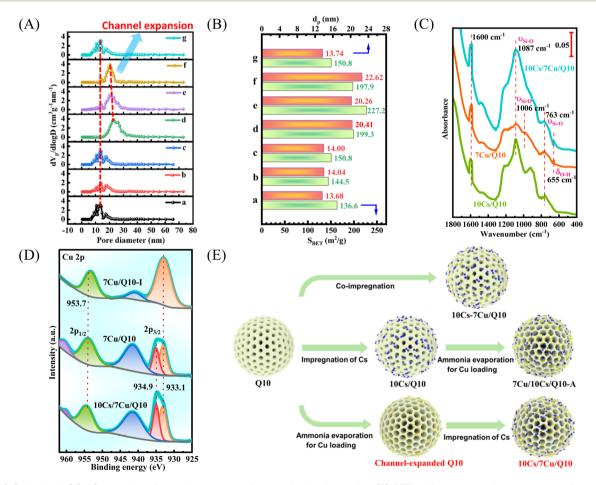
Fig. 3 (A) Calculated GCMC pore size distribution curves of as-synthesized samples. (B) BET surface area and average pore diameter of assynthesized samples: (a) 10Cs-7Cu/Q10, (b) 33Cs-22Cu/Q10, (c) 7Cu/10Cs/Q10-I, (d) 7Cu/10Cs/Q10-A, (e) 10Cs/7Cu/Q10, (f) 33Cs/22Cu/Q10, and (q) 7Cu/10Cs-Al/Q10. (C) FTIR spectra of 10Cs/Q10, 7Cu/Q10 and 10Cs/7Cu/Q10. (D) Cu 2p XPS spectra of 7Cu/Q10-I, 7Cu/Q10 and 10Cs/ 7Cu/Q10. (E) Schematic synthesis routes of 10Cs-7Cu/Q10, 7Cu/10Cs/Q10-A, and 10Cs/7Cu/Q10.
