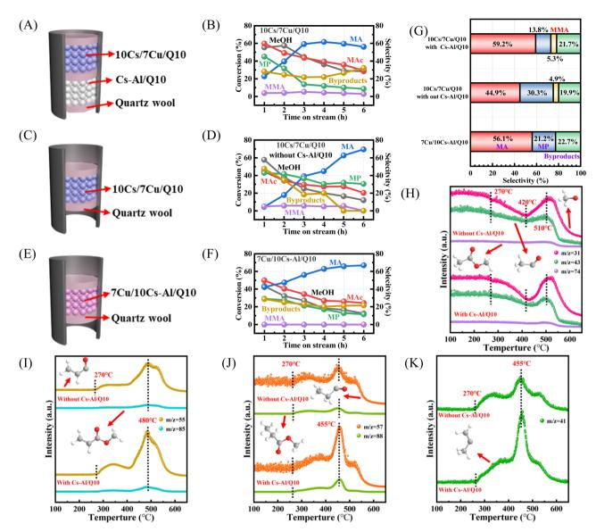
Fig. 8 Catalyst bed loading strategies and catalytic performance of (A and B) 10Cs/7Cu/Q10 with Cs-Al/Q10; (C and (D) 10Cs/7Cu/Q10 without Cs-Al/Q10; (E and (F) 7Cu/10Cs-Al/Q10. (G) Product selectivity over different samples. TPSR-MS profiles of 10Cs/7Cu/Q10 with Cs-Al/Q10 and 10Cs/7Cu/Q10 without Cs-Al/Q10: (H) signals of MeOH and MAc; (I) signals of MA; (J) signals of MP; (K) signals of MMA.
