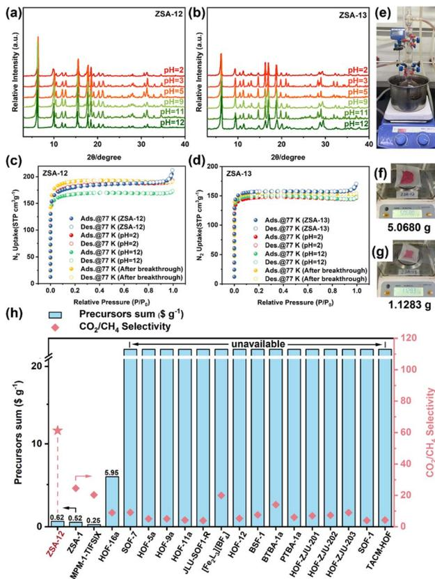
Fig. 6 Evaluation of chemical stability of ZSA-12 and ZSA-13 via (a) and (b) PXRD and (c) and (d) 77 K  $N_2$  adsorption measurements; (e) diagram of the gram-scale synthesis setup in water; samples obtained through synthesis; (f) ZSA-12, and (g) ZSA-13; (h) comparison of ZSA-12 with other HOFs in terms of separation performance and synthesis cost.
