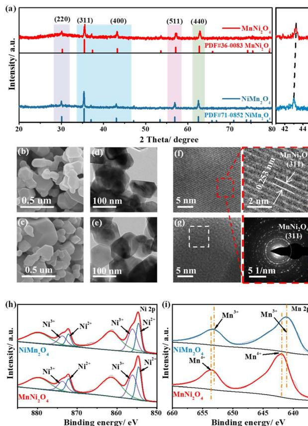
Fig. 2 (a) XRD patterns of  $\text{NiMn}_2\text{O}_4$  and  $\text{MnNi}_2\text{O}_4$ . (b) SEM image, (d) TEM image, (f) HRTEM image and SAED pattern of  $\text{MnNi}_2\text{O}_4$ . (c) SEM image, (e) TEM image, and (g) HRTEM image of  $\text{NiMn}_2\text{O}_4$ . Ni 2p (h) and Mn 2p XPS spectra (i) of  $\text{NiMn}_2\text{O}_4$  and  $\text{MnNi}_2\text{O}_4$ .
