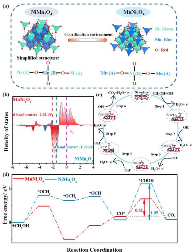
Fig. 1 (a) Structure models of  $\text{NiMn}_2\text{O}_4$  and  $\text{MnNi}_2\text{O}_4$  spinels: the transformation of  $\text{Ni}^{2+}$  from tetrahedral to octahedral coordination. (b) The partial density of states (PDOS) of  $\text{NiMn}_2\text{O}_4$  and  $\text{MnNi}_2\text{O}_4$  surfaces. (c) Diagram of the reaction process of the MOR on the  $\text{MnNi}_2\text{O}_4$ -Ni site. (d) The Gibbs free energy diagram for the MOR of  $\text{NiMn}_2\text{O}_4$  and  $\text{MnNi}_2\text{O}_4$ .
