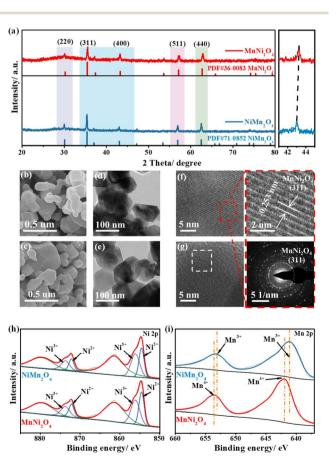
Fig. 2 (a) XRD patterns of NiMn<sub>2</sub>O<sub>4</sub> and MnNi<sub>2</sub>O<sub>4</sub>. (b) SEM image, (d) TEM image, (f) HRTEM image and SAED pattern of MnNi<sub>2</sub>O<sub>4</sub>. (c) SEM image, (e) TEM image, and (g) HRTEM image of NiMn<sub>2</sub>O<sub>4</sub>. Ni 2p (h) and Mn 2p XPS spectra (i) of NiMn<sub>2</sub>O<sub>4</sub> and MnNi<sub>2</sub>O<sub>4</sub>.
