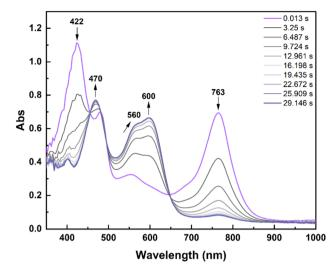
Fig. 7 Stopped-flow absorption spectral evolution upon reduction of a  $1c^{2+}$  solution (2.27  $\times$  10<sup>-5</sup> M) with a Me $_{10}$ Fc solution (2.27  $\times$  10<sup>-5</sup> M) in CH $_3$ CN. Mixing time: 10 ms. Optical path: 1 cm.
