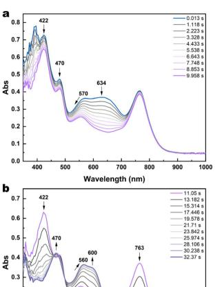
Fig. 8 Stopped-flow absorption spectral evolution upon reduction of a  $1c^{2+}$  solution (2.27  $\times$  10<sup>-5</sup> M) with a Me<sub>10</sub>Fc solution (4  $\times$  10<sup>-5</sup> M) in CH<sub>3</sub>CN (a) during the first 10 s and (b) between 11 s and 32 s. Mixing time: 10 ms. Optical path: 1 cm.
