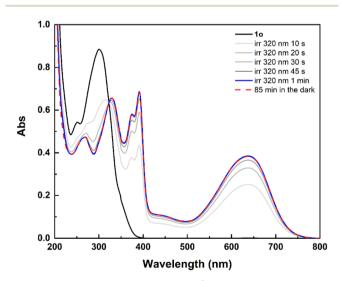
Fig. 3 Spectral evolution of 1 (1.84  $\times$  10<sup>-5</sup> M) in CH<sub>3</sub>CN under UV light irradiation (320 nm) from the open form (10, black solid line) to the photo-stationary state (blue solid line,  $\alpha_{1c}=94\%$ ). The spectrum recorded after having kept the irradiated solution in the dark at room temperature for 85 min is provided with a red dashed line. Optical path of the cuyette: 1 cm.
