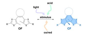
Fig. 1 Schematic representation of the multi-responsive isomerisation of diarylethenes between the open form (OF, black) and the closed form (CF, blue) showing the possible stimuli inducing the isomerisation described in the literature. X = CH, N.
