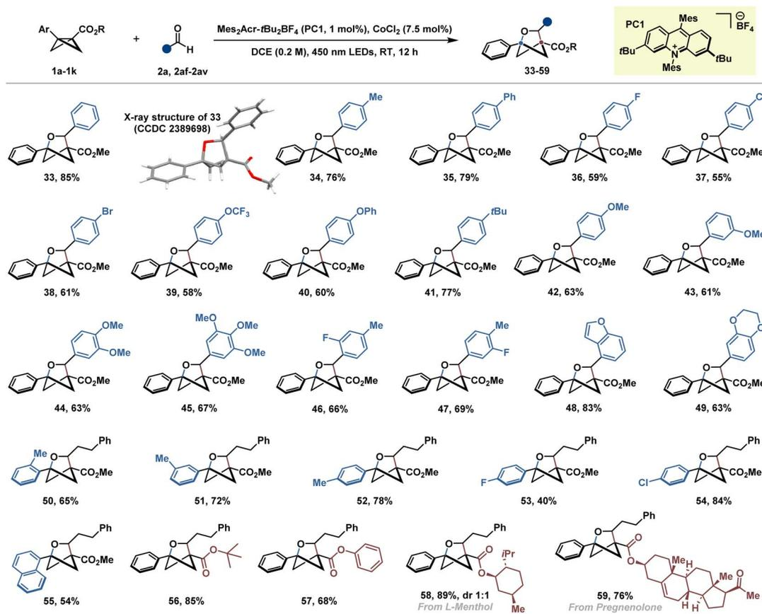
Fig. 3 Substrate scope regarding various BCBs and aldehydes. Reaction conditions:  $\text{CoCl}_2$  (7.5 mol%),  $\text{Mes}_2\text{Acr-tBu}_2\text{BF}_4$  (PC1, 1 mol%), freshly prepared BCB 1 (0.2 mmol, 2 equiv.) and aldehyde 2 (0.1 mmol, 1 equiv.) were dissolved in DCE (0.5 mL, 0.2 M). The mixture was irradiated with 30 W 450 nm blue LEDs with a cooling fan for 12 h under  $\text{N}_2$ .
