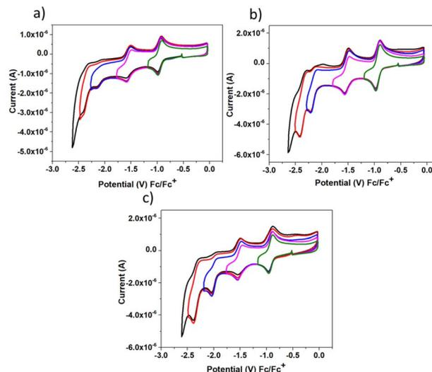
Fig. 7 CV curves of compounds **2Re** (a), **3Re** (b) and **4Re** (c). All measurements were recorded at  $100 \text{ mV s}^{-1}$  under  $\text{N}_2$  in THF with 0.1 M  $\text{TBAPF}_6$  as the supporting electrolyte.
