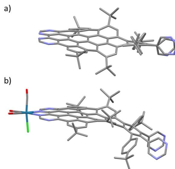
Fig. 6 Crystal structure of nanographene **2** (a) and complex **2Re** (b). Color code: carbon atoms, gray ellipsoids; chlorine atoms, green ellipsoids; nitrogen atoms, blue ellipsoids; oxygen atoms, red ellipsoids; ruthenium atoms, cyan ellipsoids. The hydrogen atoms are omitted for clarity.
