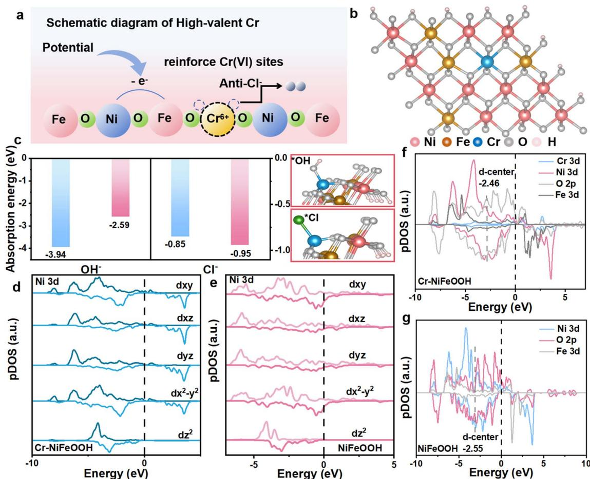
Fig. 1 (a) Design and mechanism of corrosion-resistant anodes during seawater electrolysis. Cr-NiFeLDH catalysts effectively inhibit the erosion of Cl<sup>-</sup>. (b) Optimized structural model of Cr-NiFeOOH. (c) ΔG (\*OH) and ΔG (\*Cl) of Cr-NiFeOOH and NiFeOOH. Projected density of states (PDOS) of each orbital of Ni 3d in (d) Cr-NiFeOOH and (e) NiFeOOH. PDOS in the orbital coupling of (f) Cr-NiFeOOH and (g) NiFeOOH electrocatalysts.
