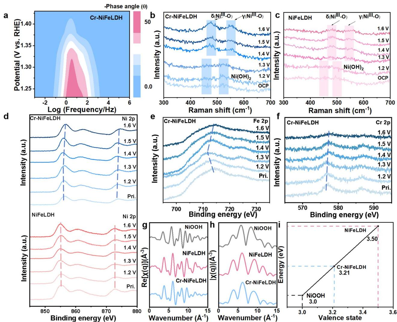
Fig. 4 (a) *In situ* Bode diagram of Cr-NiFeLDH. (b) *In situ* Raman spectra of Cr-NiFeLDH and (c) NiFeLDH. (d) Ni 2p, (e) Fe 2p, and (f) Cr 2p. XPS spectra of Cr-NiFeLDH at different voltages. (g-h) Plots in  $q$  space of NiOOH, NiFeLDH and Cr-NiFeLDH. (i) XANES valence state fitting line graph.
