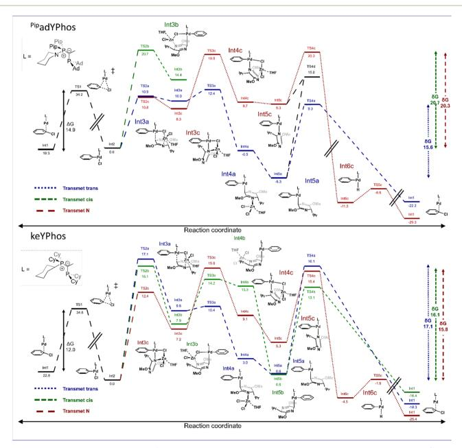
Fig. 2 Comparative energy profile (in kcal mol<sup>-1</sup>) in the arylation of valine-derived bis-lactim ether 2a and chlorobenzene 1f using PipadYPhos (top) and keYPhos (bottom). Energies (PBE0-D3/def2TZVP + LANL2TZ(f)) are given relative to the oxidative addition complex and the zincated bis-lactim ether with two coordinating THF molecules (see the ESI for details†).
