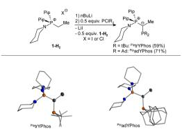
Scheme 4 Synthesis and crystals of PiptrYPhos and PipadYPhos. Molecular structures, were determined from single crystals obtained by slow evaporation from saturated C<sub>6</sub>D<sub>6</sub> solutions. Ellipsoids drawn at the 50% probability level, and hydrogen atoms omitted for clarity.
