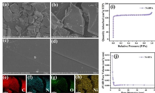
Fig. 3 The SEM images in different dimension scales of  $50\text{ }\mu\text{m}$  (a),  $10\text{ }\mu\text{m}$  (b),  $2\text{ }\mu\text{m}$  (c) and  $500\text{ nm}$  (d) in Ni-BPA. The EDS mapping of C (e), N (f), O (g) and Ni (h) elements in Ni-BPA. The  $\text{N}_2$  adsorption/desorption isotherms (i) and aperture distribution (j) of Ni-BPA.
