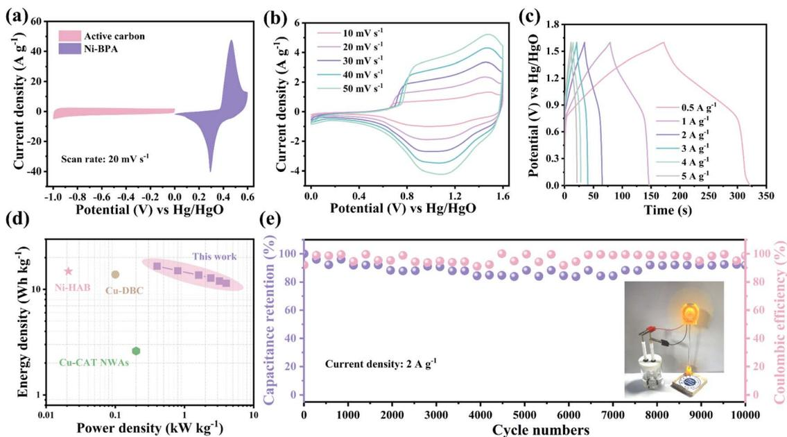
Fig. 5 (a) CV curves. (b) CV curves at various scan rates from 10 to 50  $\text{mV s}^{-1}$ . (c) GCD curves at various current densities from 0.5 to 5  $\text{A g}^{-1}$ . (d) Ragone plot and (e) cycling performance (inset shows a small fan) of the Ni-BPA//AC device.
