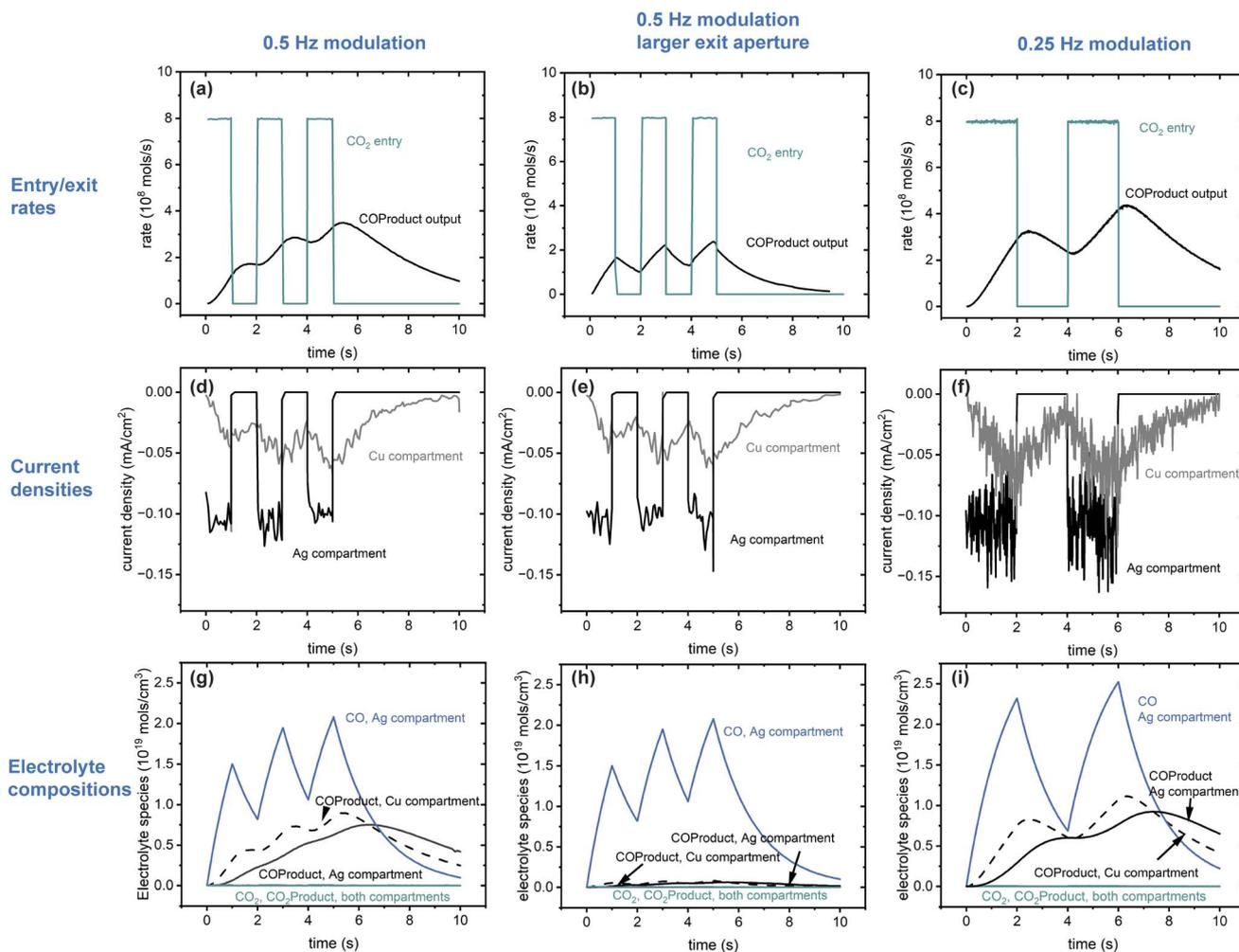
Fig. 5 Line plots of key characteristics of the cascading system for the 3 cases in Table 2. (a)–(c) comparison of the  $\text{CO}_2$  entrance rate and COProduct exit rate, (d)–(f) comparison of the catalytic currents in the Ag and Cu compartments as calculated on a catalytic surface area of  $0.05 \mu\text{m}^2$  at the same location in them, (g)–(i) comparison of the electrolyte compositions.
