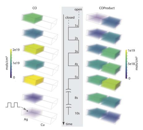
Compartment contents as a function of time point in the aperture open-close modulation cycle, for a total time of 10 s.
