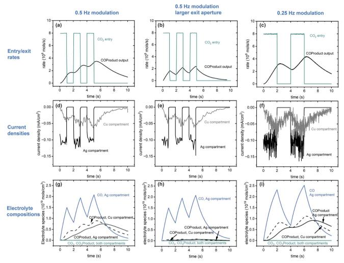
Fig. 5 Line plots of key characteristics of the cascading system for the 3 cases in Table 2. (a)–(c) comparison of the  $CO_2$  entrance rate and COProduct exit rate, (d)–(f) comparison of the catalytic currents in the Ag and Cu compartments as calculated on a catalytic surface area of 0.05  $\mu$ m<sup>2</sup> at the same location in them, (g)–(i) comparison of the electrolyte compositions.
