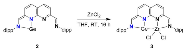
Scheme 3 Complexation of \text{ZnCl}_2 to the empty pocket of 2 , yielding 3 .
