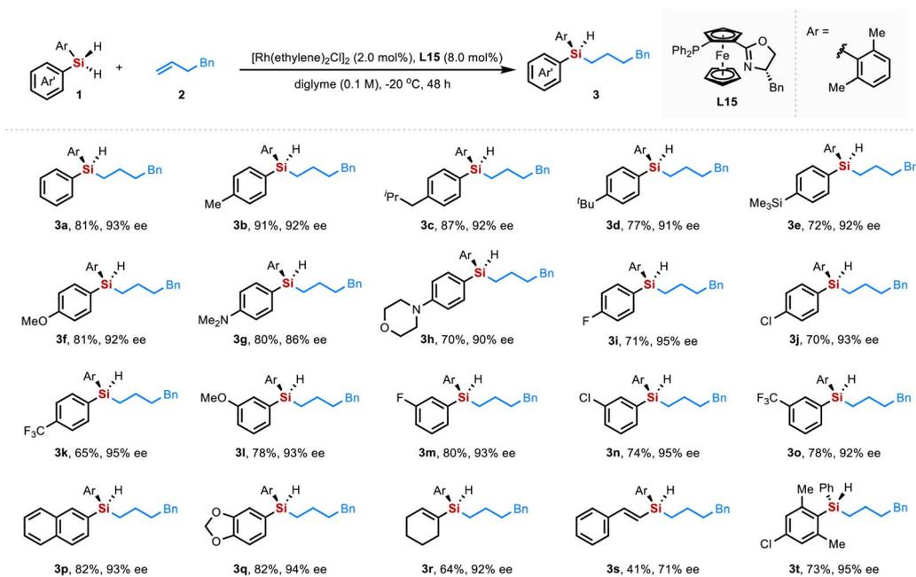
**Scheme 3** Scope of dihydrosilanes<sup>a,b</sup>. <sup>a</sup>Reaction conditions: **1** (0.2 mmol), **2** (31.8 mg, 0.24 mmol),  $[\text{Rh}(\text{ethylene})_2\text{Cl}]_2$  (1.6 mg, 2.0 mol%), **L15** (8.4 mg, 8.0 mol%), diglyme (2.0 mL),  $-20^\circ\text{C}$ , 48 h,  $\text{N}_2$ . <sup>b</sup>Isolated yield; the ee value was determined by chiral HPLC analysis.
