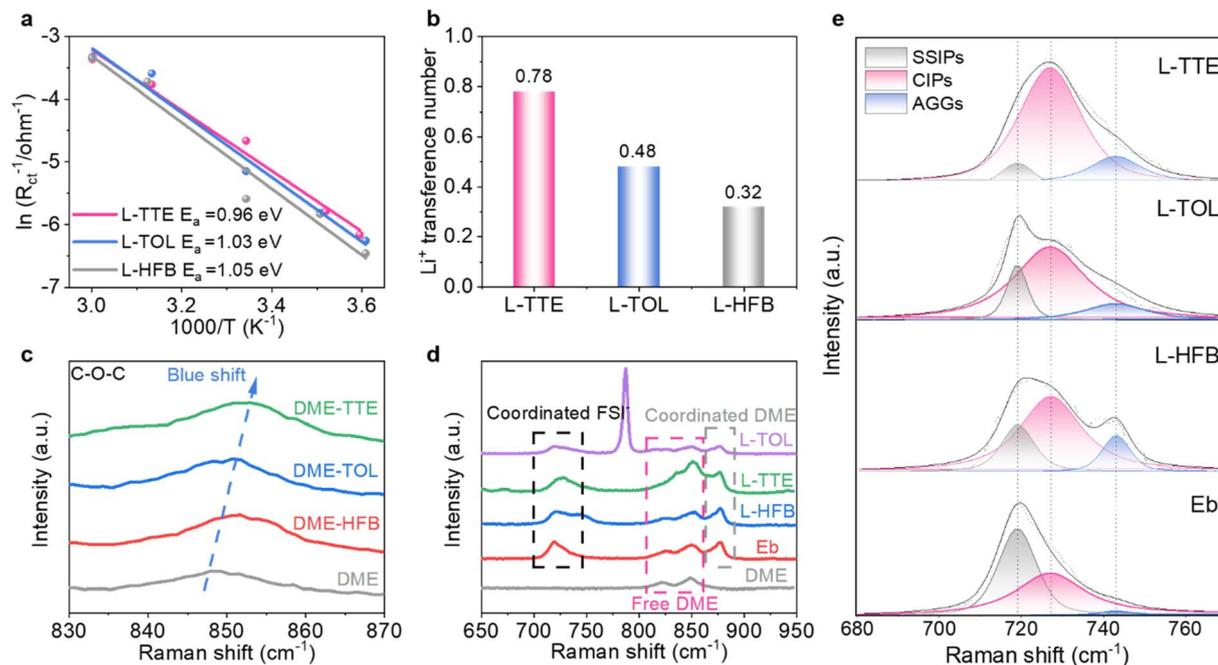
Fig. 2 (a) Activation energies calculated from the Arrhenius equation. (b)  $\text{Li}^+$  transference numbers of different electrolytes. (c) Raman spectra of DME and DME/diluent. (d) Raman spectra of electrolytes. (e) Raman spectra and fitting results of electrolytes in the range of  $680\text{--}770\text{ cm}^{-1}$ .
