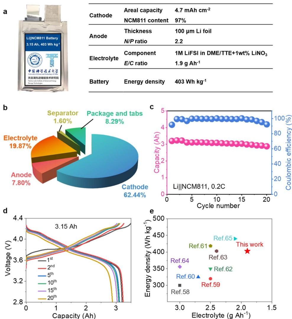
Fig. 5 (a) Schematic illustration of pouch cell parameters. (b) Weight ratios of cell components. (c) Cycle performance of the 403 Wh kg<sup>-1</sup> Li||NCM811 pouch cell. (d) Capacity–voltage plots of the pouch cell. (e) Comparison of lithium-metal pouch cells in previous reports and this work.
