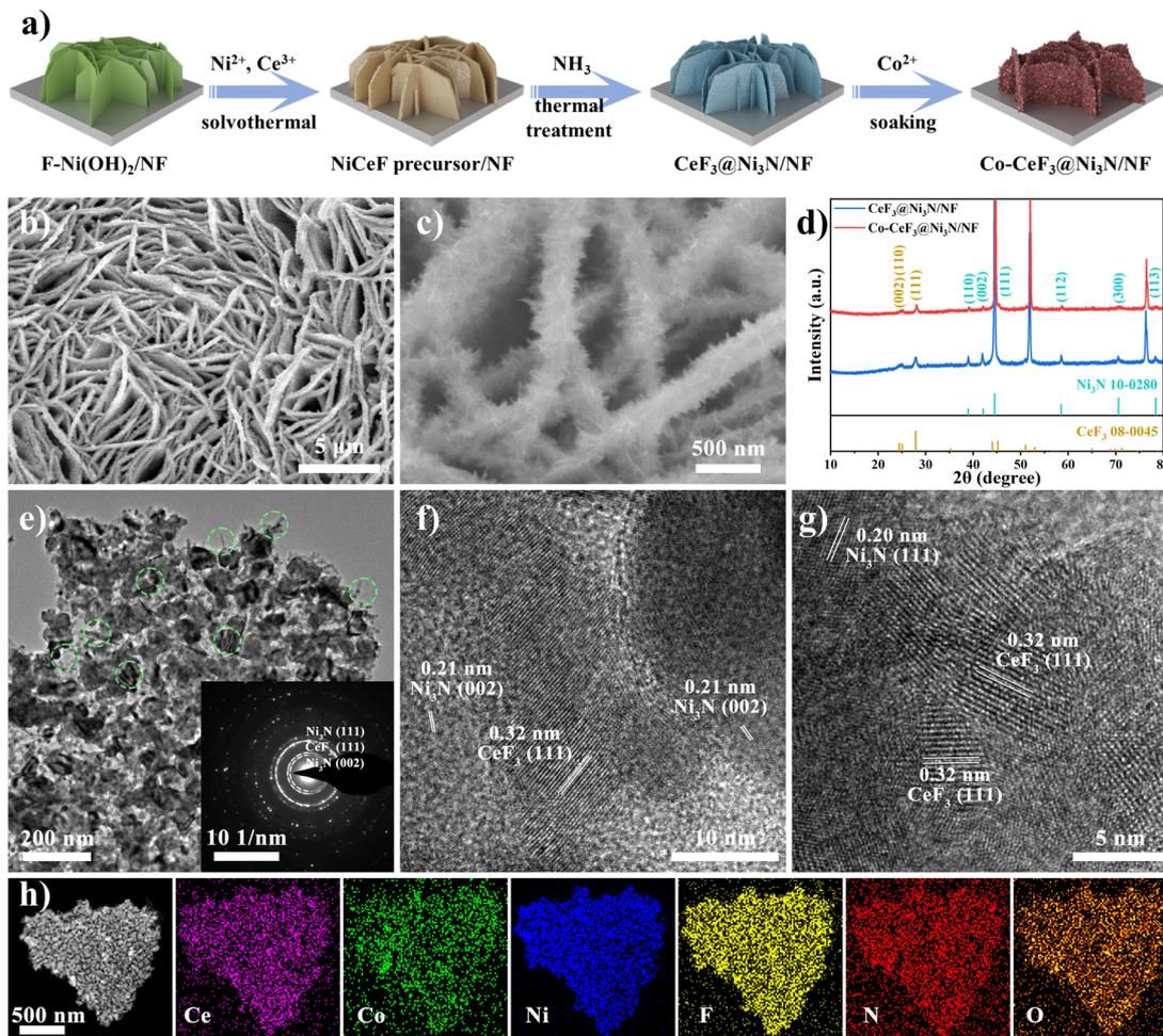
Fig. 1 (a) A schematic illustration of the synthetic procedure for Co-CeF<sub>3</sub>@Ni<sub>3</sub>N/NF. (b) and (c) SEM images of Co-CeF<sub>3</sub>@Ni<sub>3</sub>N/NF. (d) XRD patterns of CeF<sub>3</sub>@Ni<sub>3</sub>N/NF and Co-CeF<sub>3</sub>@Ni<sub>3</sub>N/NF. (e)–(g) TEM images and the SAED pattern of Co-CeF<sub>3</sub>@Ni<sub>3</sub>N. (h) A HAADF-STEM image and corresponding EDX mapping of Co-CeF<sub>3</sub>@Ni<sub>3</sub>N.
