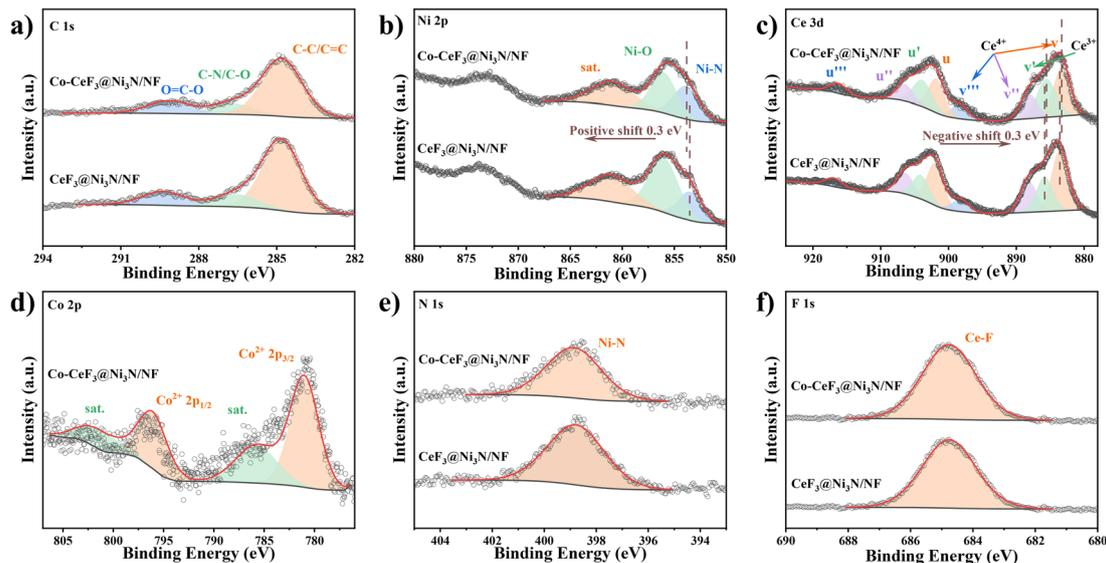
Fig. 2 (a) C 1s, (b) Ni 2p, (c) Ce 3d, (d) Co 2p, (e) N 1s, and (f) F 1s XPS spectra of Co-CeF<sub>3</sub>@Ni<sub>3</sub>N/NF and CeF<sub>3</sub>@Ni<sub>3</sub>N/NF.
