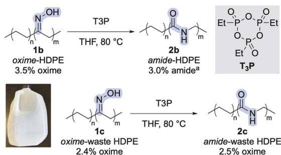
Scheme 1 Beckmann rearrangement of additional oxime-polyethylenes with T3P. <sup>a</sup>The small difference in percent functionality could be attributed to the inherent error of determining percent functionalization of this level of groups in a polymer by <sup>1</sup>H NMR spectroscopy.
