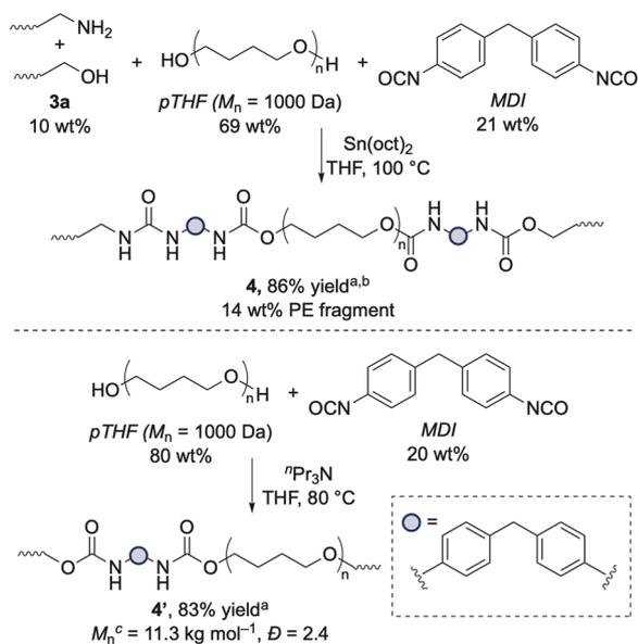
**Scheme 2** Synthesis of PUUs through polymerization of alcohol- and amine-terminated LDPE fragments with MDI and *p*THF. <sup>a</sup>Yield with respect to mass. <sup>b</sup>We were unable to characterize the resulting material by gel-permeation chromatography (GPC) because of its insolubility in THF at 35 °C, DMF at 55 °C, or 1,2,4-trichlorobenzene at 135 °C. <sup>c</sup>Absolute molecular weight was calculated following detector calibration with a single narrow poly(styrene) standard.
