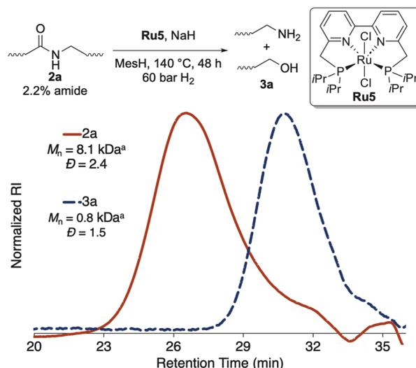
Fig. 2 Hydrogenolysis of amide linkages in amide-LDPE. <sup>a</sup>Molecular weight with respect to polyethylene standards.
