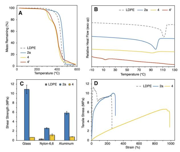
Fig. 3 Summary of materials properties. (A) TGA curves of unmodified LDPE, polymer 2a, PUU 4, and PU 4'. (B) DSC traces of unmodified LDPE, polymer 2a, PUU 4, and PU 4'. (C) Lap-shear tests of unmodified LDPE, polymer 2a, and PUU 4 as interlayers with aluminum, nylon-6,6, and glass substrates. The mode of failure for all lap-shear tests was determined to be adhesive failure. (D) Stress-strain curves of unmodified LDPE, polymer 2a, and PUU 4. Strain rate  $= 50 \text{ mm min}^{-1}$ .
