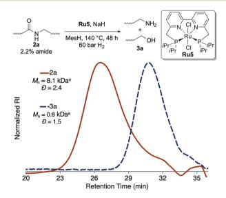
Fig. 2 Hydrogenolysis of amide linkages in amide-LDPE. <sup>a</sup>Molecular weight with respect to polyethylene standards.
