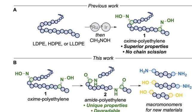
Fig. 1 (A) Prior work: synthesis of oxime-polyethylene. (B) This work: Beckmann rearrangement of oxime-polyethylene to form in-chain amide linkages and hydrogenolysis to create precursors for new materials.
