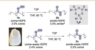
Scheme 1 Beckmann rearrangement of additional oxime-polyethylenes with T3P. <sup>a</sup>The small difference in percent functionality could be attributed to the inherent error of determining percent functionalization of this level of groups in a polymer by <sup>1</sup>H NMR spectroscopy.
