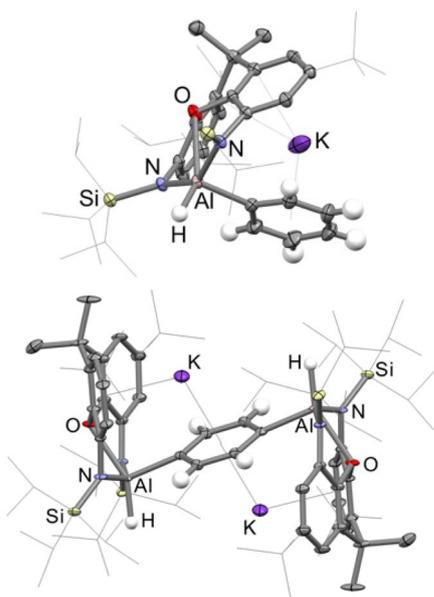
Fig. 2 Structures of **2** and **3** as determined by X-ray crystallography. Displacement ellipsoids set at the 50% probability level. Most hydrogen atoms have been omitted and selected organic groups have been shown in wireframe for clarity.
