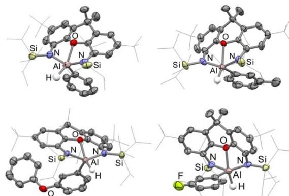
Fig. 7 Structures of 5 (top-left), 6 (top-right), 7 (bottom-left) and 9-H (bottom-right) as determined by X-ray crystallography.  $[\text{K}(\text{18-crown-6})]$  cations and most hydrogen atoms have been omitted for clarity. Displacement ellipsoids set at the 50% probability level and selected organic groups have been shown in wireframe.
