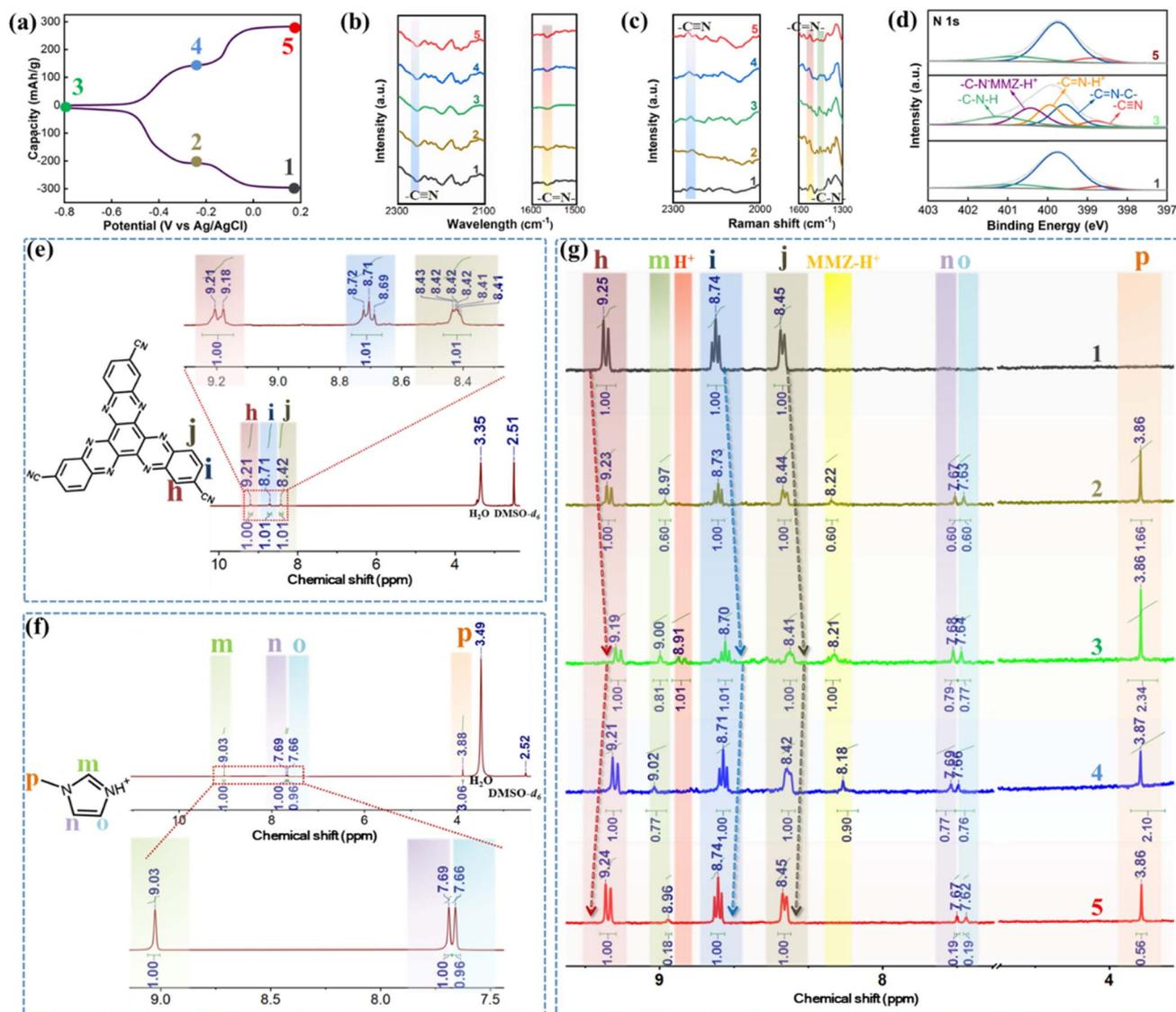
Fig. 4 Energy storage mechanism of HATN-3CN in 50M-10S electrolyte. (a) Indication of different charge and discharge states. (b) *Ex situ* FT-IR spectra. (c) *In situ* Raman spectra. (d) *Ex situ* XPS spectra of N 1s.  $^1\text{H}$ -NMR spectra of pure HATN-3CN powder (e) and the imidazolium ion (MMZ/ $\text{H}_2\text{SO}_4 = 1:2$ ) (f). (g) *Ex situ*  $^1\text{H}$ -NMR spectra. Note: the solvents used for the  $^1\text{H}$ -NMR spectra were  $\text{DMSO}-d_6$  in e-g.
