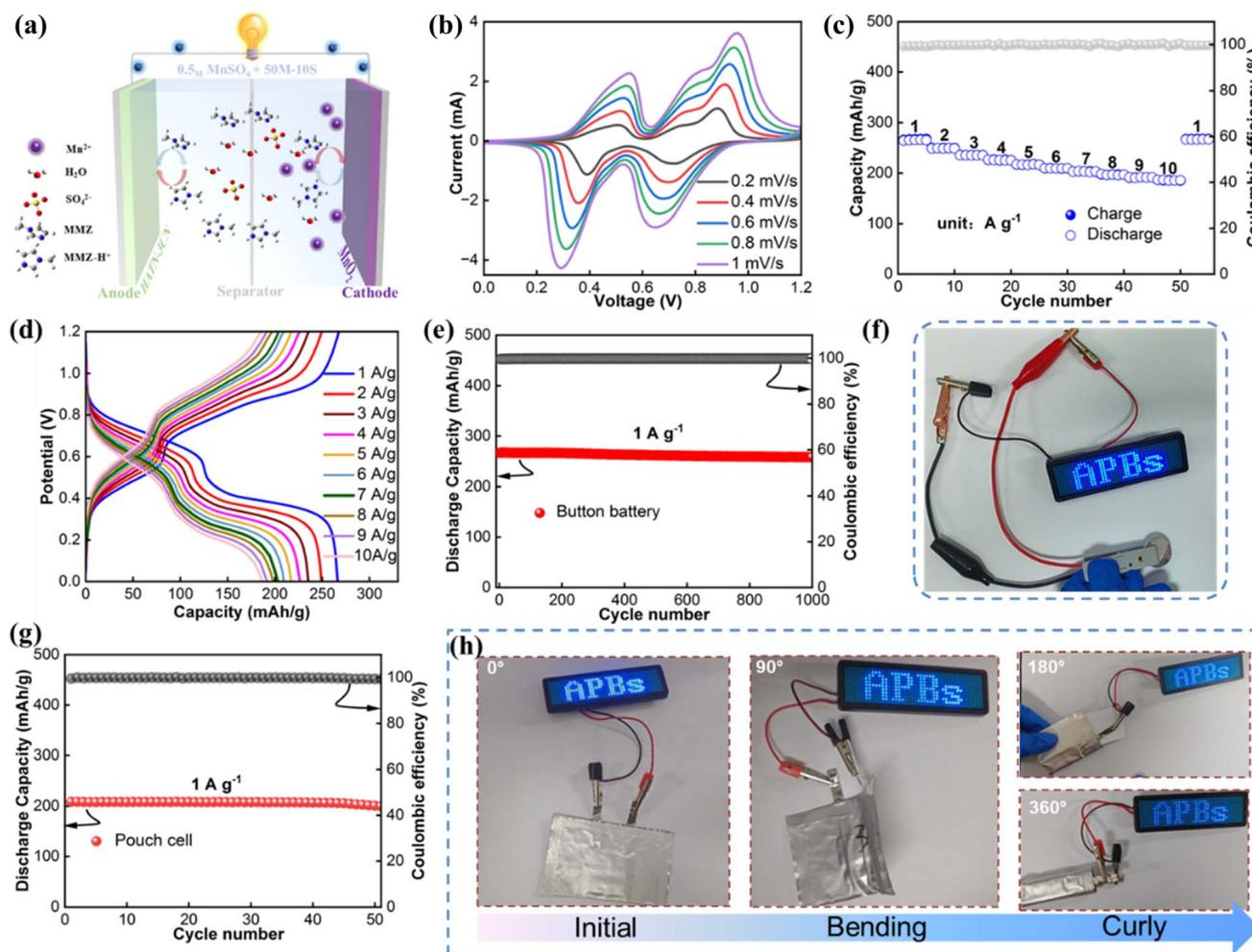
Fig. 6 Electrochemical performance of the HATN-3CN//MnO<sub>2</sub> full battery. (a) Schematic illustration of the full battery. (b) CV curves at different scan rates from 0.2 to 1 mV s<sup>-1</sup>, (c) rate performance, (d) charge–discharge curves, (e) cycling performance at 1 A g<sup>-1</sup> and (f) optical image of an LED screen powered by a button-type battery. (g) Cycling performance at 1 A g<sup>-1</sup> and (h) optical image of an LED screen powered by the pouch cell.
