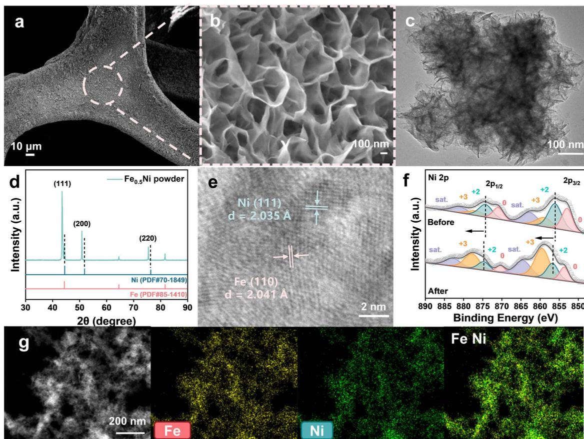
Fig. 2 Morphology characterization. (a) and (b) SEM images of as-deposited  $\text{Fe}_{0.5}\text{Ni}/\text{CF}$  catalyst. (c) TEM image of  $\text{Fe}_{0.5}\text{Ni}$ . (d) XPS spectra of Ni 2p for  $\text{Fe}_{0.5}\text{Ni}$  prior to and post electrolysis at 1.38 V vs. RHE. (e) HRTEM image of  $\text{Fe}_{0.5}\text{Ni}$ . (f) XRD pattern of  $\text{Fe}_{0.5}\text{Ni}$  powder. (g) HAADF-STEM image and corresponding elemental mappings of Fe and Ni for  $\text{Fe}_{0.5}\text{Ni}$ .
