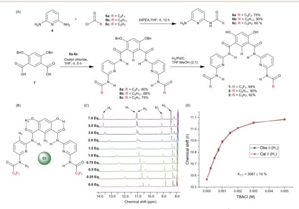
Fig. 2 (A) Synthesis of transporters 1-3. (B) Chemical structure of transporter 1 complexed to chloride. (C)  $^1H$  NMR titration spectra for 1 (2.5 mM in THF- $d_8$ ) with stepwise addition of TBACl in THF- $d_8$ . Protons assigned in panel B, and the equivalents of added TBACl are shown on the stacked spectra. (D) The plot of chemical shift ( $\delta$ ) of proton H<sub>1</sub> vs. concentration of TBACl added for transporter 1, fitted to a 1:1 binding model using BindFit.
