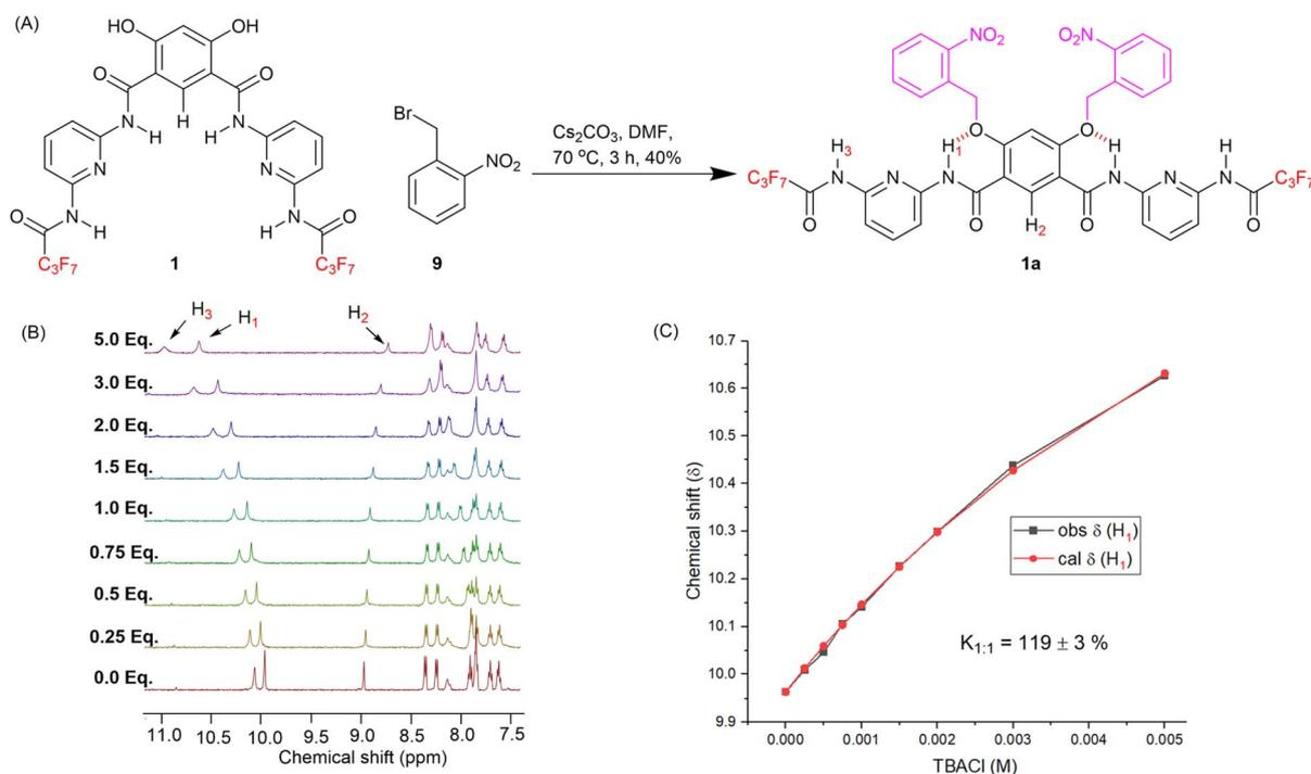
Fig. 4 (A) Synthesis of pro-transporter 1a. (B)  $^1H$  NMR titration spectra for 1a (2.5 mM in  $THF-d_8$ ) with stepwise addition of TBACl in  $THF-d_8$ . The equivalents of added TBACl are shown on the stacked spectra. (C) Plot of chemical shift ( $\delta$ ) of  $H_1$  proton vs. concentration of TBACl added for transporter 1, and fit to a 1:1 binding model.
