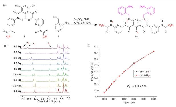
Fig. 4 (A) Synthesis of pro-transporter  ${\bf 1a}$ . (B)  $^1{\bf H}$  NMR titration spectra for  ${\bf 1a}$  (2.5 mM in THF- $d_8$ ) with stepwise addition of TBACl in THF- $d_8$ . The equivalents of added TBACl are shown on the stacked spectra. (C) Plot of chemical shift ( $\delta$ ) of H<sub>1</sub> proton vs. concentration of TBACl added for transporter  ${\bf 1}$ , and fit to a 1:1 binding model.
