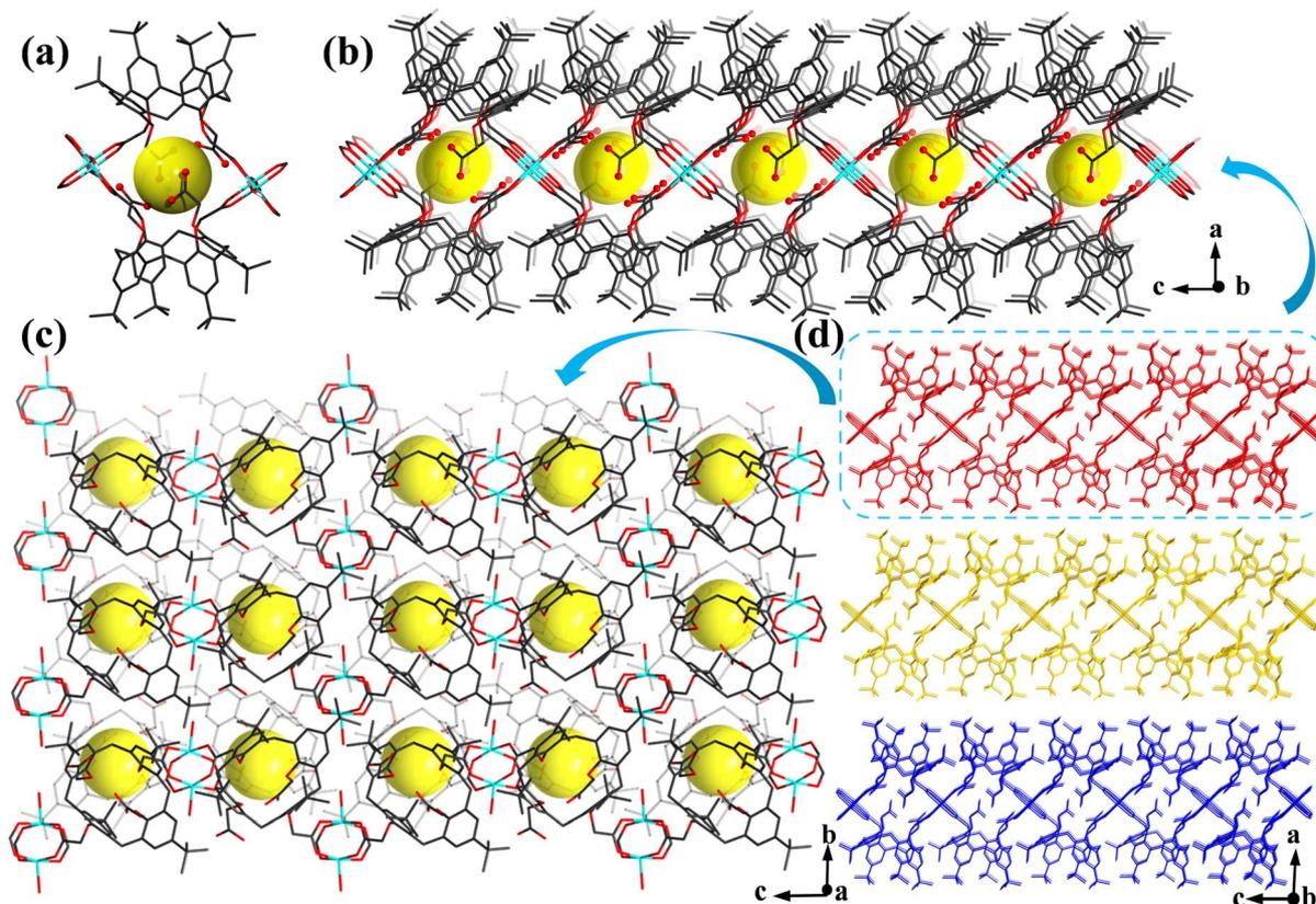
Fig. 1 (a) View of the cage-like secondary building unit in **Cu-MOF-COOH**. Atom color codes: cyan, Cu; red, O; dark gray, C. (b and c) View of the 2D structures in **Cu-MOF-COOH**. (d) The 3D structure of **Cu-MOF-COOH**.
