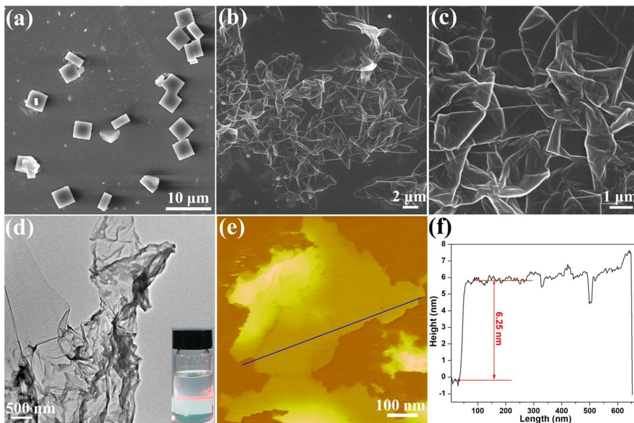
Fig. 2 (a) SEM image of the square-shaped bulk **Cu-MOF-COOH**. (b and c) SEM images of **Cu-MOF-COOH** nanosheets. (d) TEM image of **Cu-MOF-COOH** nanosheets; inset: photograph of the Tyndall effect of **Cu-MOF-COOH** nanosheet suspension. (e) AFM image of **Cu-MOF-COOH** nanosheets. (f) Height profile, color-coded blue, is measured along the corresponding track shown in (e).
