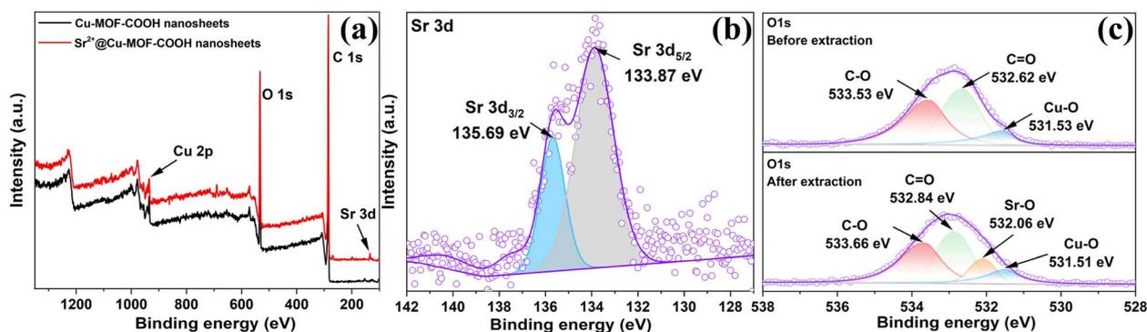
Fig. 4 (a) XPS survey spectrum of Cu-MOF-COOH nanosheets (contrast of Sr<sup>2+</sup> extraction). (b) High-resolution XPS spectra of Sr 3d (after Sr<sup>2+</sup> extraction) and (c) O 1s (before and after Sr<sup>2+</sup> extraction).
