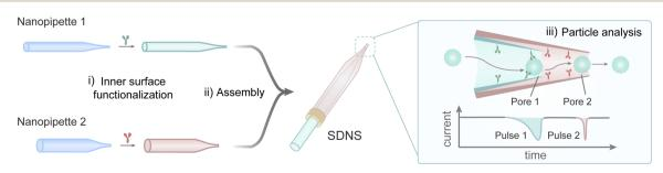
Fig. 1 Schematic diagram of the main fabrication process of SDNS for single-particle analysis.
