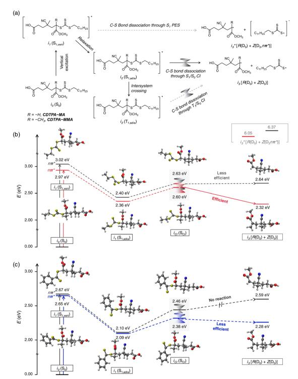
Fig. 2 (a) Plausible photoinduced C-S bond dissociation pathway of CDTPA-MA and CDTPA-MMA. Plausible energy profiles for the photoinduced C-S bond dissociation of (b) CDTPA-MA (grey), CDTPA-MMA (red) and (c) CPADB-MA (grey), CPADB-MMA (blue).
