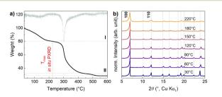
Fig. 4 (a) TGA data of S1, heating rate 5 K min<sup>-1</sup> under synthetic air atmosphere (flow rate 70 mL min<sup>-1</sup>) (black) and the derivation of the TGA data (light green). (b) Temperature dependent (30–220 °C) *in situ* PXRD measurements including selected reflection indices using an open capillary of S1. Dotted lines are included to indicate the peak shifts.
