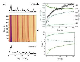
Fig. 8 (a) In situ PXRD measurement of open capillary of vacuum dried S1 over time (RH of  $25\pm5\%$ ). Evolution of (b) lattice parameter changes, volume changes, and (c) the unit cell angle changes during the rehydration of NTU-9-d by ambient atmosphere.
