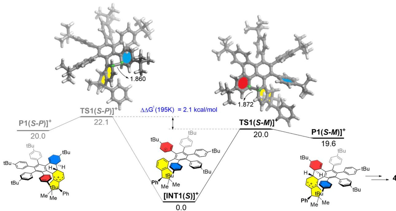
Fig. 2 Computed reaction profiles for the key Scholl cyclization step occurring at the beginning of the graphitization process. Relative free energies ( $\Delta G$ , at 195 K) and bond distances are given in  $\text{kcal mol}^{-1}$  and angstroms, respectively. All data were computed at the CPCM-RI-B3LYP-D3(BJ)/def2-SVP level.
