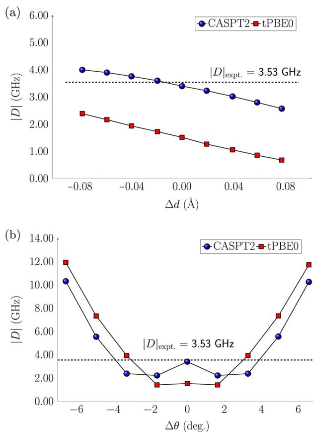
Fig. 3 CASPT2 and tPBE0 axial parameter  $|D|$  of  $\text{Cr}(o\text{-tol})_4$  complex for (a) the Cr–C symmetric stretching, and (b) the C–Cr–C scissoring normal modes. The equilibrium bond angle is  $\theta = 104.9^\circ$ , and the equilibrium bond distance is  $d = 1.98$  Å.
